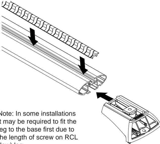
Note: In some installations it may be required to fit the leg to the base first due to the length of screw on RCL (low) leg.
