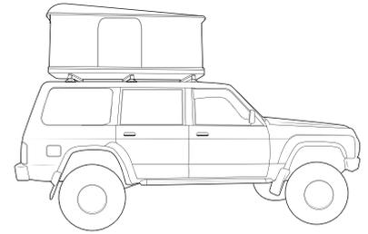
When these roof racks are to be used on a vehicle that is driven off sealed roads, the manufacturer maximum roof load rating (to be found in the vehicles User Manual) should be **divided by 1.5**. Do not forget to subtract the complete crossbar system weight from your maximum carrying capacity.
