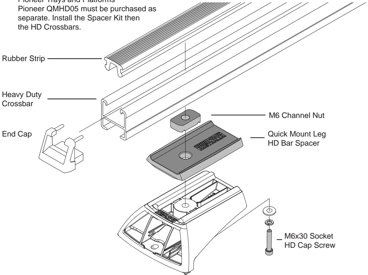
To fit Legs to Pioneer Trays/ Platforms, positioned wide on vehicle, QMPS10 must be purchased as separate. Install the Spacer Kit then the Tray/ Platform.
