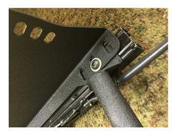
E) Side mounts. The R-9173/4 seat track adaptors are designed to work with either the R-906X line of side mounts (if using Recaro sliders) or the R-907X and R-975X line of side mounts (if bolting the side mount directly to the seat track adapter). The side mounts you use should be selected by the width of the seat you're installing in the car. Use the hardware included with the side mounts to bolt the side mount to the slider or seat track adapter.
