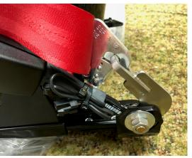
The (included) outboard lap belt mount attaches at the same location as the factory outside lap belt, reusing the stock bolt. If you're also using the R-1150 harness bar, there's no need to install this lap belt mount as the functionality is built into the R-1150's downtube base.
