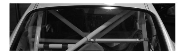
Step 4: Reference belt harnesses manufacturer's installation instructions for mounted the shoulder harnesses to the R-1040. It is common practice to cross shoulder belts to prevent slippage.
