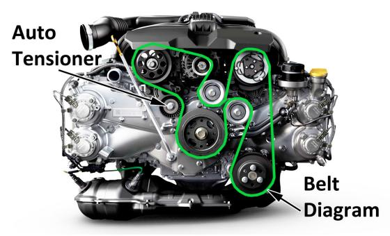
Above Diagram for FB Engine (2012+ Impreza), FA engine (BRZ/FR-S) has similar roughting excpet upper middle pulley is missing.
