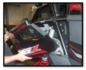
3. It is required that you trim the inner fender to gain clearance for the rear shocks once the lift kit is installed. See illustration on where to trim the inside of the rear panels.
