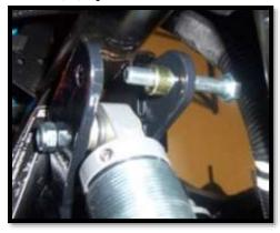
15. Attach the shock to the lift brackets using the same bolt.
