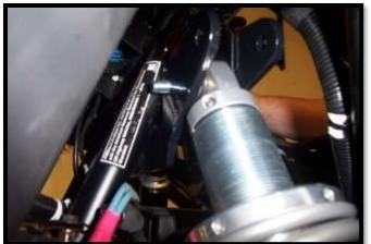
10. Secure the bracket loosely to the bolt with a 10mm lock nut.
