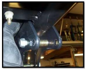
14. Attach the shock to the brackets using the same 12mm x 75mm bolt.
