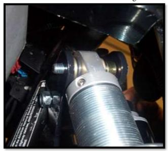
16. Now attach the inner lift bracket to the bolt and secure it loosely using a 10mm lock nut.
