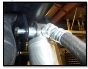
16. Now connect the rear inner lift plate loosely with the 12mm lock nut.
