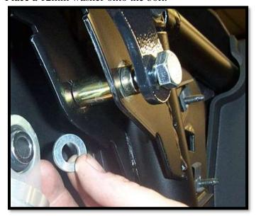
10. Next attach the (77R) rear inner plate onto the bolt and loosely fasten with 12mm lock nut.
