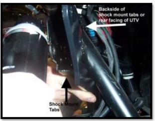
5. Before you insert the second front lift bracket, you need to rotate the shock revisors on both shocks. This will allow for bracket clearance. Rotate to the front inside of the frame on both sides. NOTE: The orientation for the illustrations is the front right side of UTV.
