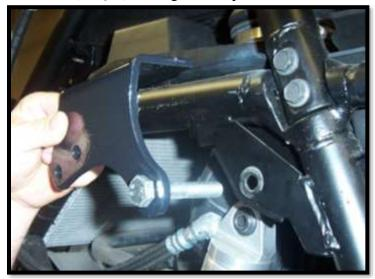
7. Next place an (AA) spacer onto the bolt and then insert it into the shock mount tab.
