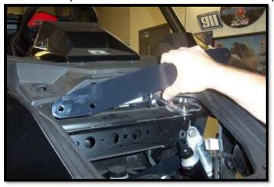
7. Insert a 10mm x 70mm bolt through the bracket and then place a 10mm flat washer onto the bolt.
