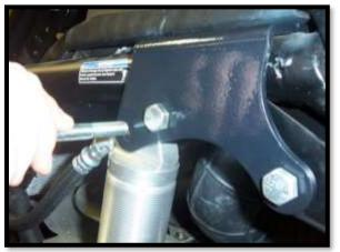
15. Place the (30I) spacer onto the bolt next to the shock eye and rear inner lift bracket
