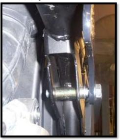
9. Place a 12mm washer onto the bolt.
