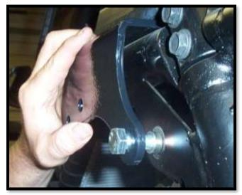
8. Place a (O) spacer between the shock mount tabs and finish inserting the bolt though the tabs.
