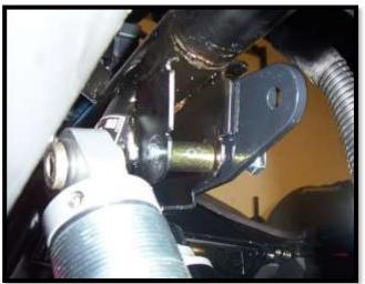
9. Place a 10mm washer onto the bolt, then place the bracket onto the bolt.
