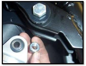
11. Insert a 12mm x 75mm bolt through the rear outer plate.
