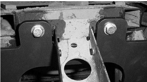
NOTE: Make sure to reconnect the bottom of the plastic support bracket to the frame using the stock hardware.
