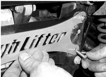
**Note:** The bolts in the photo are Hex head and were replaced with button head bolts.
