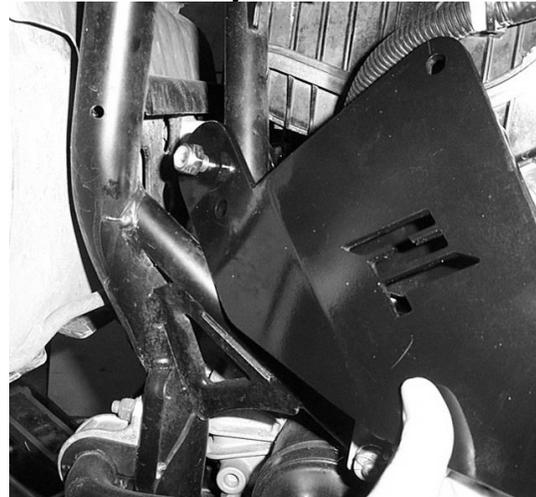
6. Now connect the inner bracket to the frame by inserting the 10x80mm bolt through the frame shock mount tab, then through the bracket. Insert the **Spacer 39C** between the plate and the shock mount tab. Push the bolt through the spacer and tab.
