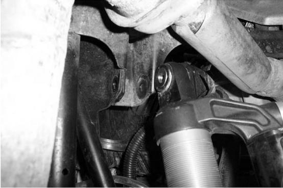
4. Starting from the passenger's side, rear right from the seated position; insert the inner right bracket into place **between the shock mount tabs**. But first place a 10x55mm bolt through the lower portion of the bracket. It is going to be very difficult to insert this bolt if you do not install it first. Now insert the bracket into place.
