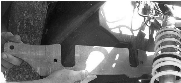
10. Connect the bracket to the frame by placing it on the bolts and fasten it using the 10mm lock nuts provided.
