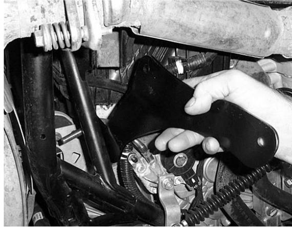
5. Connect the outer rear right bracket to the bolt and secure it loosely with the 10mm nut.
