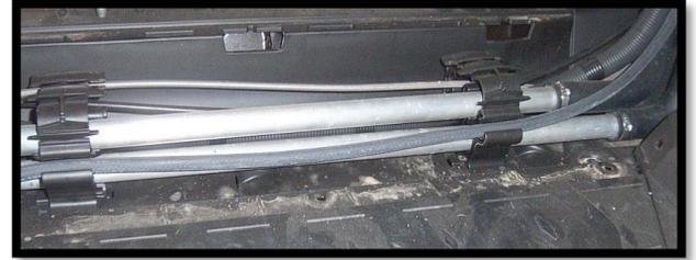
e. Disconnect the rear supply brake line from the master cylinder. Remove it and the rear brake lines. **(It is optional to simply cut them for faster removal since they will not be reused)**
