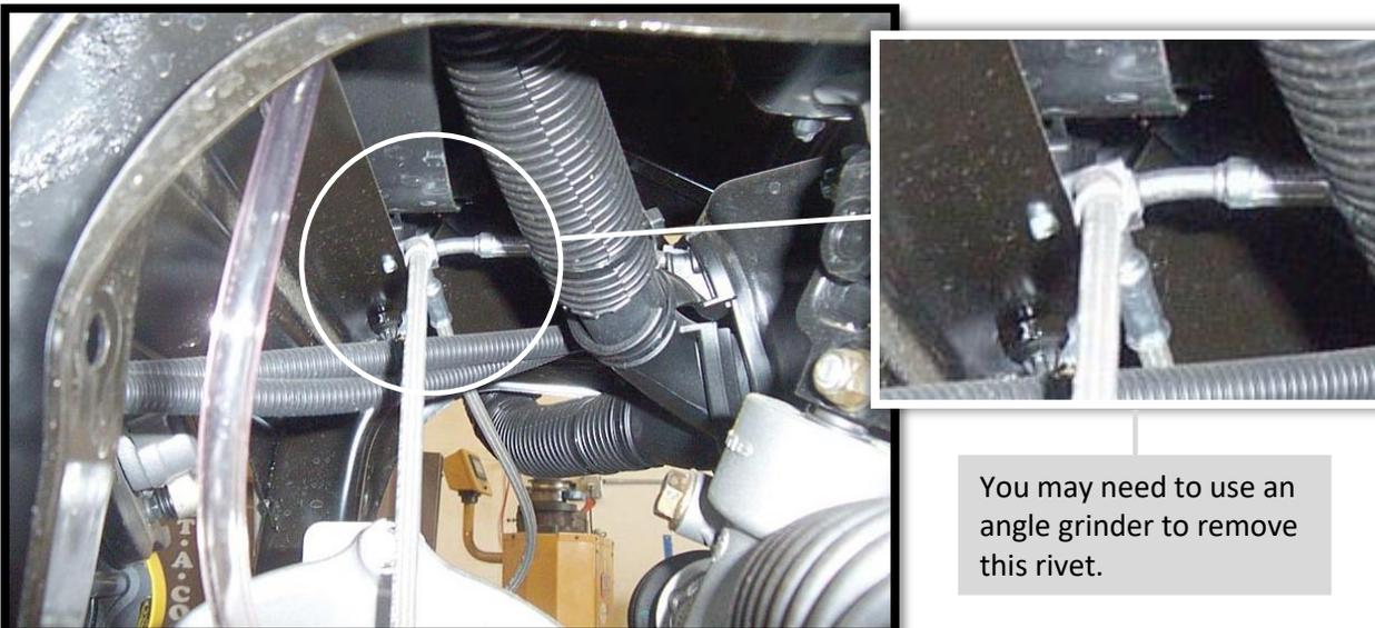
You may need to use an angle grinder to remove this rivet.
