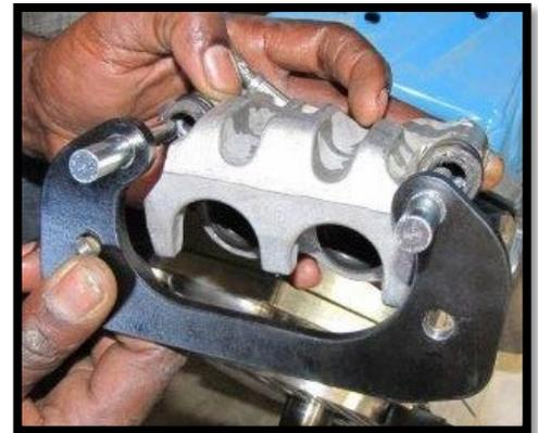
On the portal box, the brake caliper will be relocated to the FRONT. Because of this...
