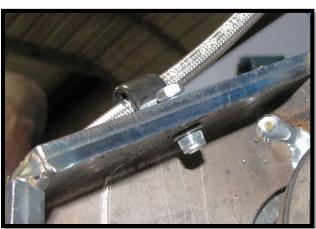
h. Use the factory A-arm clips and the supplied **zip ties** to reposition the brake lines, then fasten the brake line back to the caliper. **Make sure there's no binding in the lines, even at full turn.**
