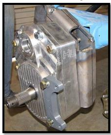
d. Loosely fasten the all six bolts with 1/2" flat washers and 1/2" lock nuts. Recheck all parts that were used and make sure everything fits correctly, and then go ahead and tighten and torque all bolts. (3/4)[105 ft lbs]
