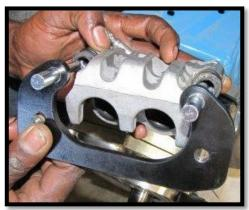
On the portal box, the brake caliper will be relocated to the FRONT. Because of this...
