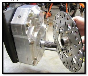
b. Slide on the supplied **30mm lock washer**, followed by the **30mm spindle castle nut**. (46mm) [**Min 120 ft lbs**] Tighten the castle nut further if needed to align grooves with holes in the spindle for the cotter pin. Install the supplied **cotter pin**. Both ends of the cotter pin must be folded.
