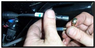
d. Install the new **(45X) 48" FRONT LEFT** brake line to the banjo bolt. Run the line back through the frame and to the (DR) side hub.
