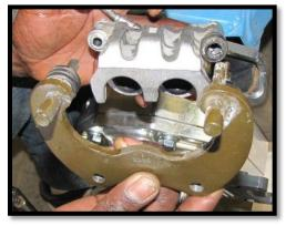
c. Find the new rear brake caliper hanger bracket **PGLC-BCB-85X.** Apply **LOCTITE (BLUE)** to the pins and fasten them to the bracket. [73 ft lbs] Then insert it into the brake caliper.
