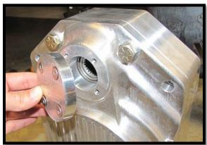
c. Find the caliper mounting bracket **PGLC-BCB-115N** and place it in the corresponding fitted <u>front</u> section of the portal box. Then insert a **1/2** x **4-3/4**" **bolt** and **1/2**" **washer** into the bracket holes & box.
