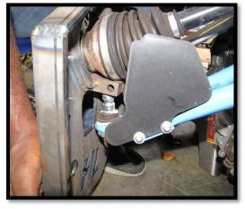
c. Insert the drive shaft into the backing plate. Then place the upper ball joint into the upper ball joint mount bracket. Fasten it with the factory hardware. (15mm)[50 ft lbs]
