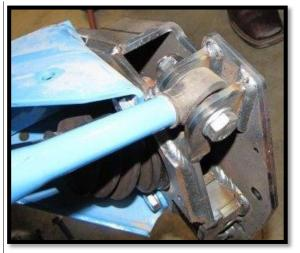
c. Slide a **12mm washer** onto a **12mm x 65 bolt**. Use it to reattach the lower radius bar. Secure it using a **12mm washer** and **12mm lock nut**. (18mm)[90 ft lbs]
