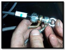
c. Install the new (107A) 54" FRONT RIGHT brake line to the banjo bolt. Run the line back through the frame and to the (PA) side hub.
