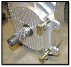
d. Slide a 1/2" flat washer onto (4) 1/2 x 4-1/2" bolts and insert them into the remaining four holes of the box.
