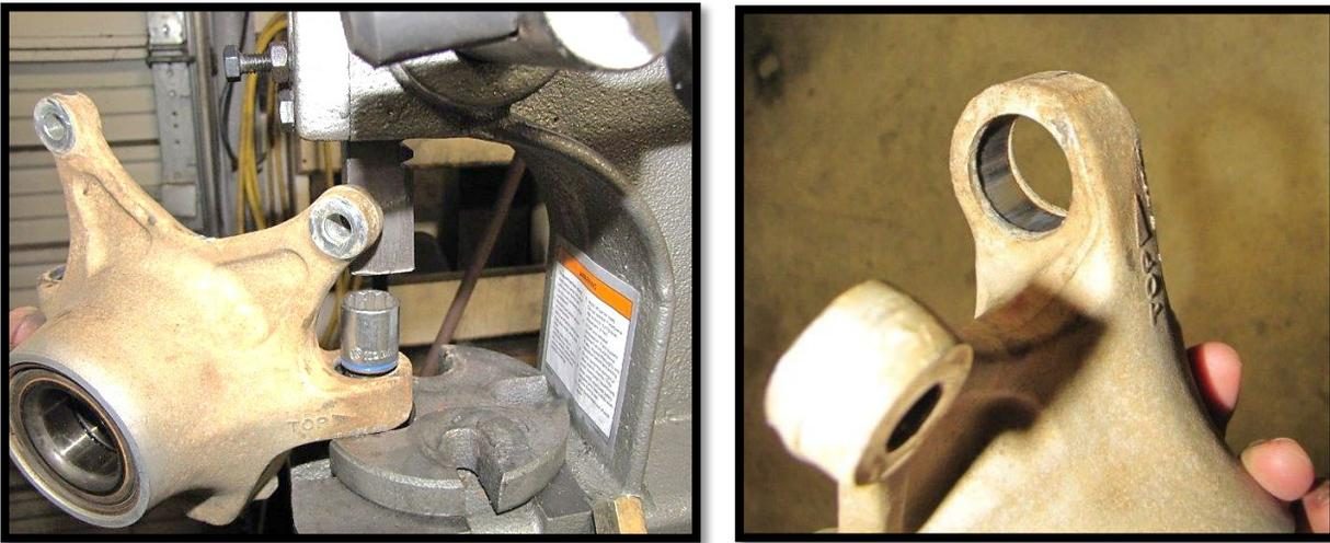
d. Inspect the radial joints for excessive wear or damage. If they show significant signs, they need to be replaced.
