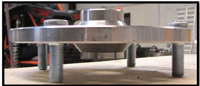
e. Once the studs are pressed in, place (4) ½" brake rotor spacers PGLC-ROTOR-SP over the tapped holes.
