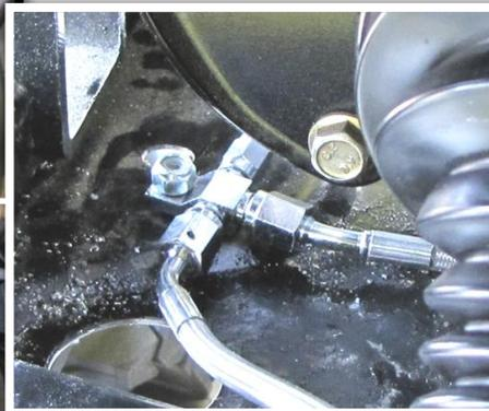
i. If you are installing 6" portals, you must route the brake lines down the inside of rear lower arms to gain enough slack.
