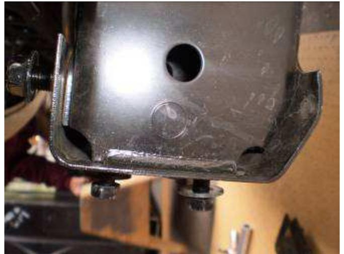
12. If you are unable to get the cutoff wheel along the entire weld then it may be necessary to break the ends loose with a hammer and chisel.
