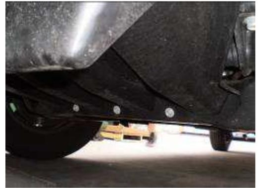
4. Once the skid plate is removed you will have access to 2 bolts on each side that hold another bumper support piece to the frame. Remove these 2 bolts from each side.
