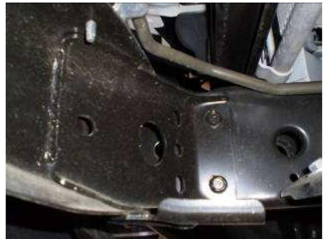
5. Once the Skid Plate is removed you should be able to unbolt the main bumper structure. There are 3 bolts on each frame rail that are accessed through the front of the bumper. You will see a 4th bolt on each side that does not actually hold the bumper on, but part of the inner bumper structure. You can remove this bolt as well if you would like.
