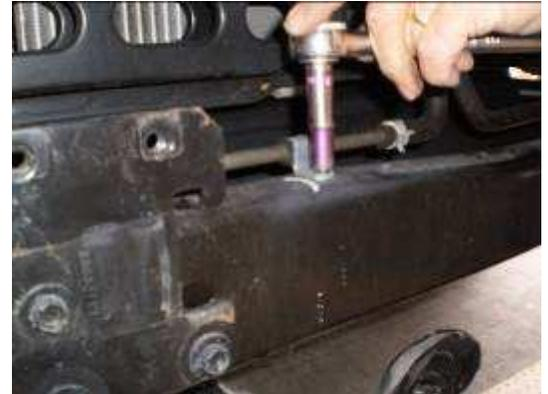
8. Take off the 2 bolts holding the cooler lines to the crossmember.
