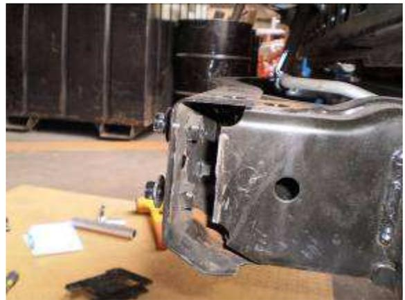
13. It is now time to install your Aluminess Bumper. Have a friend help you hold the bumper up to the vehicle and line it up with the frame. Use the provided half inch bolt to go through the side plate of the bumper and through the large hole in the side of the frame.
