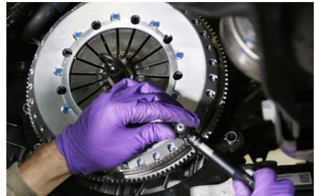
24. Remove the alignment tool. The tool should remove smoothly. If not, the discs may have shifted during tightening. If necessary, loosen the screws and repeat steps 23-24 until the alignment tool removes smoothly.
