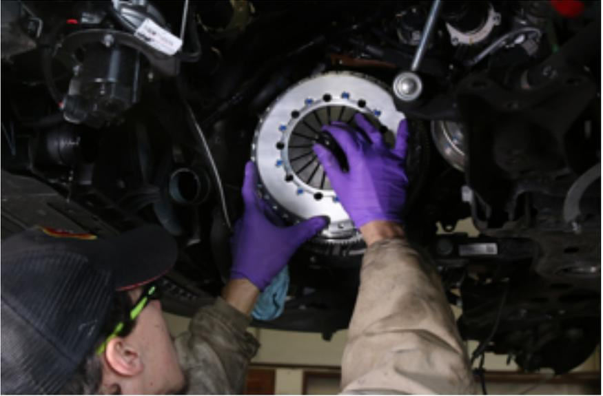
26. Be sure to remove the flywheel locking mechanism before reassembly of the vehicle.
