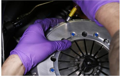
21. Taking care to check that the alignment tool is centered in the crank shaft, using the included T-25 bit, tighten each of the pressure plate screws by one full turn in a crisscross fashion.
