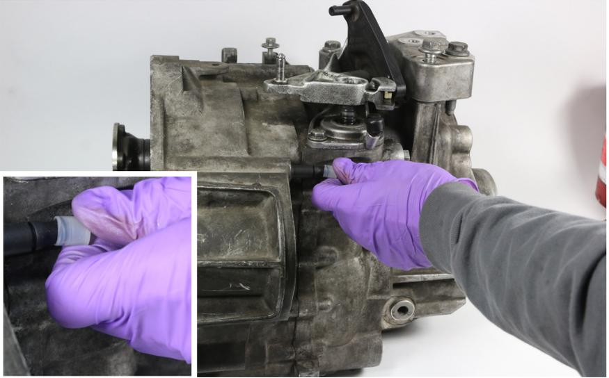
2a. Secure the funnel to the hydraulic bearing feed line.
