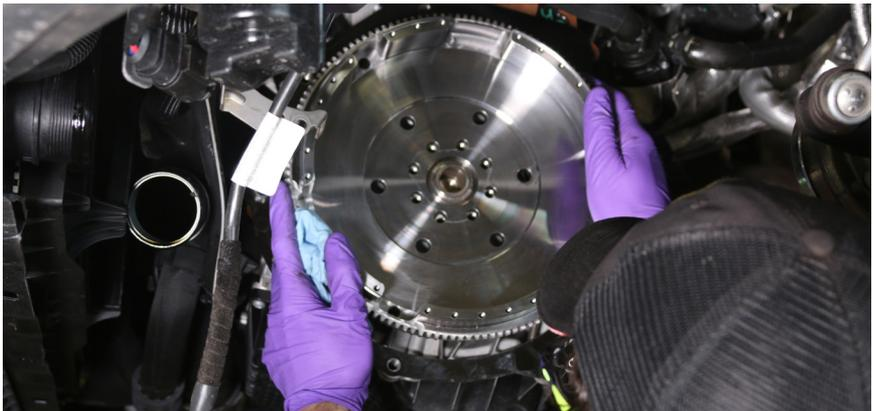
8. Install the crank bolts finger-tight only. Do not tighten them yet.
