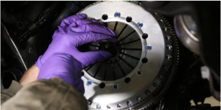
23. Tighten each of the pressure plate screws by another full turn in a criss cross fashion. Repeat until there is no gap between the pressure plate and the flywheel.
