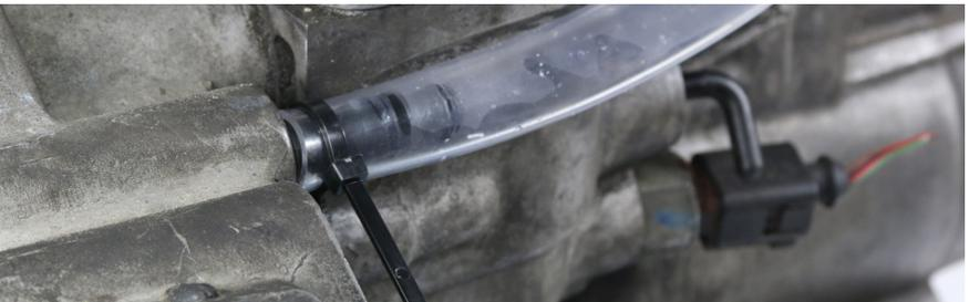
3a. Pour brake fluid into the funnel that is connected to the hydraulic bearing.
