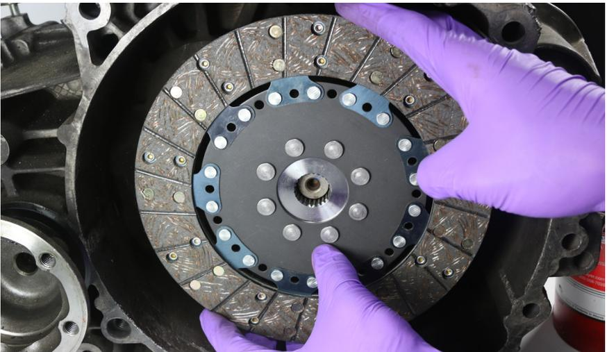
14. Remove the excess grease from the disc and input shaft, leaving only a VERY thin layer on the splined section of the shaft. Any excess grease will spin off the input shaft and contaminate the friction material; causing slipping, chatter, glazing, and other engagement issues. Contaminated friction material is not covered under warranty.
