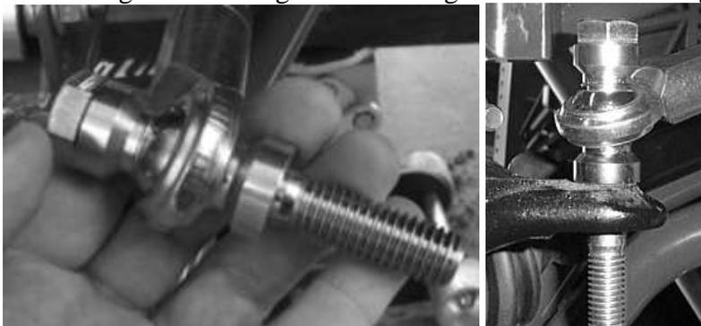
13. Place the 1/2" washer and 1/2" lock nut on the bolt and torque tight.
