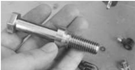
12. Insert the new 1/2 x 3 1/4" hex bolt. Slide the bolt through the alignment bushing, then the heim joint and then through another alignment bushing. Insert the bolt through the knuckle assembly.
