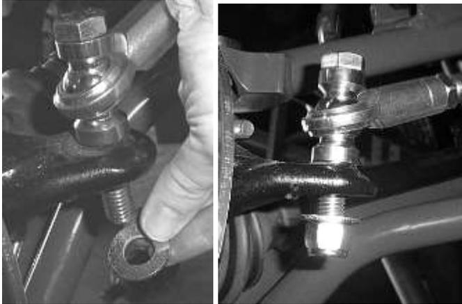
14. If you have not already done so, reconnect the bottom of the shock to the upper arm using the stock hardware.
