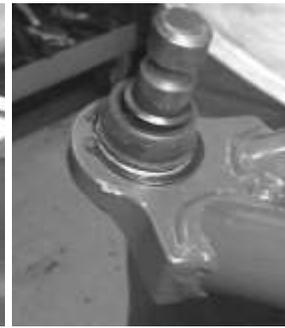
7. Use the factory nuts and bolts to connect the new control arms to the RUV frame. You will have left and right upper and lower control arms.
