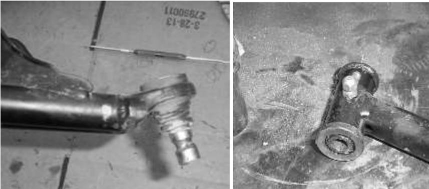
5. Install the grease fitting into the new arms before installation. **DO NOT OVER TORQUE THE FITTINGS.**
