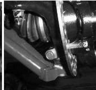
9. Remove the stock tie rod end and connect the new heim joint provided.
