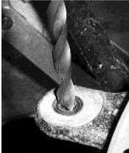
11. Once you have drilled the hole, use the 1/2 x 3 1/4" hex bolt and the two high alignment bushings and connect the heim joint to the knuckle.
