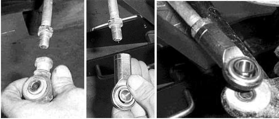
10. To connect the new heim joint to the knuckle assembly you will need to use a 1/2" drill bit and drill a larger hole where the tie rod connects to the knuckle.
