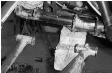
4. Remove the bushings, sleeves, and ball joints from the stock control arms. You will need to reuse these in the new kit.
