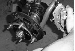
3. Remove the upper and lower control arms from the RUV. Disconnect from the frame, shock, sway-bar, and hub assembly. **NOTE: You do not need to remove the tie rod from the hub.**
