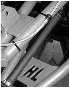
15. Reconnect the sway-bar to the control arm using the factory hardware.
