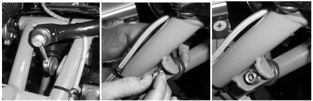
16. If you have not already done so, reconnect the bottom of the shock to the upper arm using the stock hardware.
