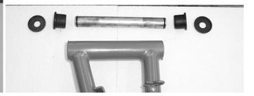
5. Now reinstall the bushings, sleeves, and ball joints into the new arms. If you place some grease on them it makes the installations easier.
