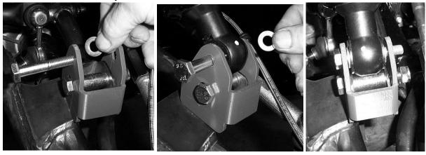
5. Secure the bracket, shock and washers to the UTV using a 10mm x 65mm bolt and 10mm lock nut.
