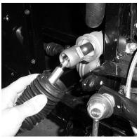
9. Place the steering stop clips between the inner tie rod joint and the rack and pinion. **You will insert two steering stops per side!** It is a tight fit, so you may have to force them on to ensure that the spacers stay in place.
