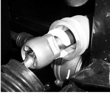
10. Pull boot back over the ball joint and steering stop and refasten with 11" zip tie. Be sure to verify the zip tie is tight so prevent material from getting into the boot.
