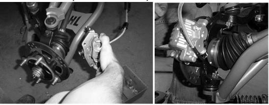
14. Connect the brake lines to the control arms using the zip ties provided.
