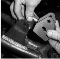
3. Insert the 10mm x 65mm bolt through the lift bracket, shock tabs, and spacer. Loosely secure the bracket using a 10mm lock nut.
