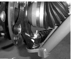
13. Next reconnect the calipers to the hub assembly.
