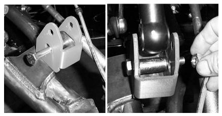
4. Next connect the bottom of the shock to the lift bracket. You will need to place a 10mm washer on either side of the shock eye.
