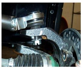
15. Connect the sock to the upper control arm using the factory hardware.
