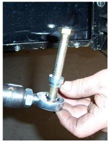
20. Now insert the large alignment cone into the hub assembly and then insert the bolt through the cone.
