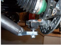
14. Now connect the upper control arm to the frame and hub assembly. Fasten the nut tight and secure with cotter pin.
