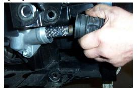
9. Place the steering stop clips between the inner tie rod joint and the rack and pinion. **You will insert one thin 55Z per side!** It is a tight fit, so you may have to force them on to ensure that the spacers stay in place.
