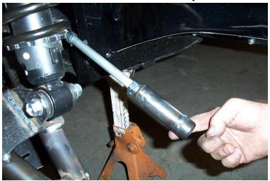
18. Included in the kit is a new heim joint and jam nut. Connect the jam nut to the heim joint. Connect the heim joint to the tie rod extension.
