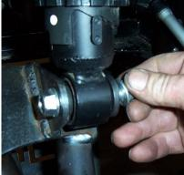
16. Remove the factory tie rod end but leave the jam nut attached to the tie rod.
