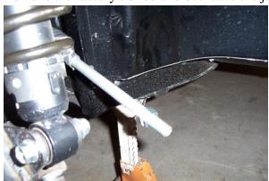
17. Connect the tie rod extension to the factory tie rod.
