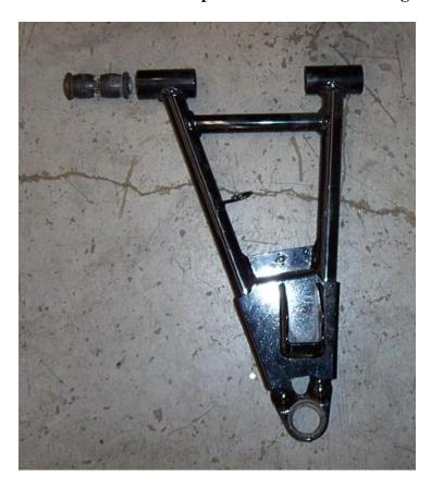
5. Now reinstall the bushings and ball joints into the new arms. If you place some grease on them it makes the installations easier. **Use a vise for the bushings and a press for the ball joints.**
