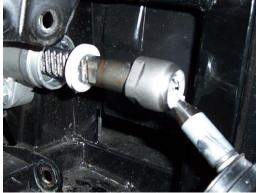
10. Pull boot back over the ball joint and steering stop. Slide replacement clamp onto the tie rod and boot. Secure the boot to the rack and pinion with clamp.
