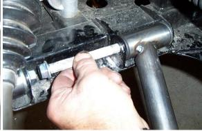
13. Connect the lower arm to the knuckle assemble. Fasten the nut tight and secure with cotter pin.
