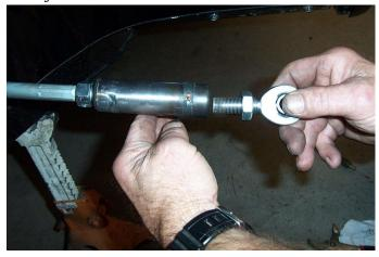
19. Included in the kit are  $\frac{1}{2}$ " x 4-1/2" hex bolts, small alignment cones and large alignment cones. Place a small alignment cone onto the bolt. Next insert the bolt through the heim joint.
