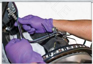
Now that your lighting wheel ring is fully installed, you must wire each ring to the ORACLE Rocker Switch that is provided. A wiring diagram is provided below to insure proper installation.
