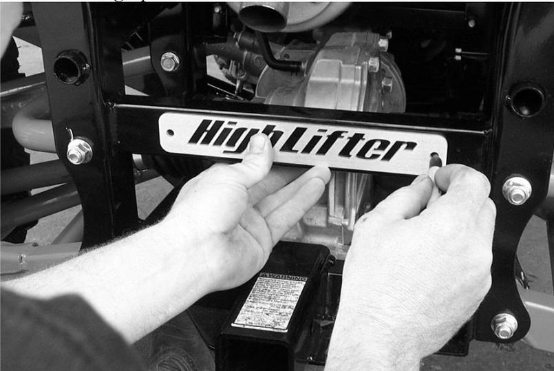
3. Using a small drill bit, drill a pilot hole for the self tapping screws.
