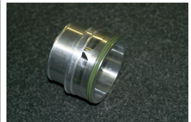
26. Install factory seal on NEUSPEED billet hose coupling then lightly oil.
