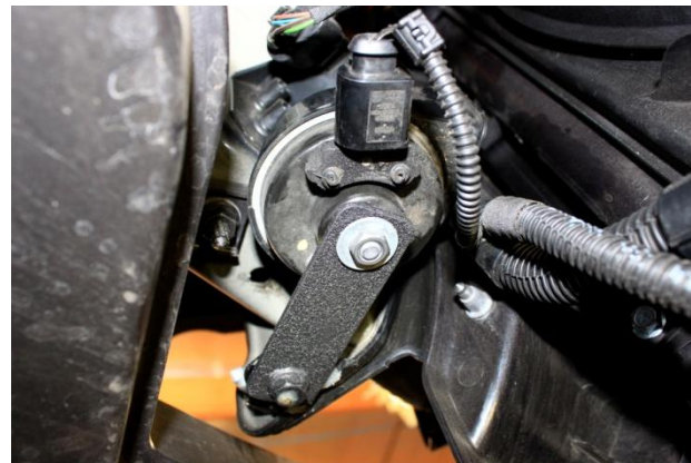
15. Using a 13mm wrench, unbolt left-side horn from its bracket. Remove OE bracket and using supplied bracket, remount horn toward inside of frame rail as pictured.
