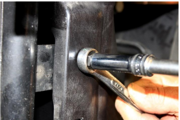
19. Hold body from turning with 14mm wrench then push and turn setting bolt with 10mm socket until Nutsert crimps firmly in hole. Remove tool.
