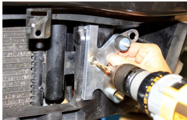
17. Attach both left and right side intercooler mounts into existing square holes in radiator core support, then lock down, now drill 1/4" thru core.
