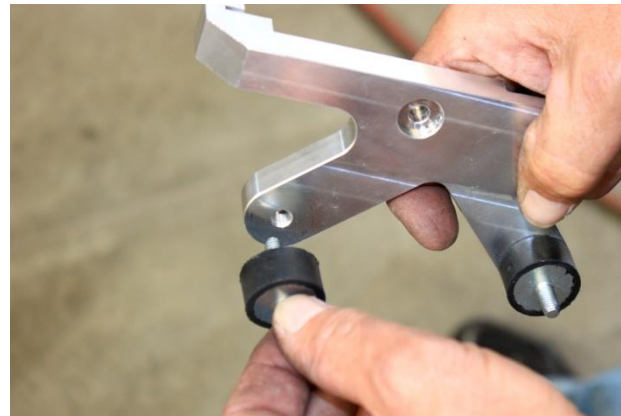
16. Install and tighten rubber isolators into billet intercooler mounting brackets.
