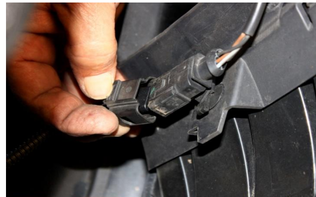
8. Before pulling front bumper completely off, disconnect both side marker lamp connections and both fog light or running light connections.
