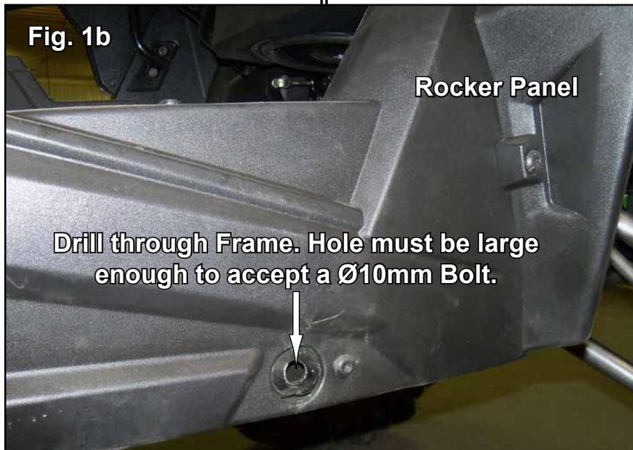
**Drill through Frame. Hole must be large enough to accept a Ø10mm Bolt.**
