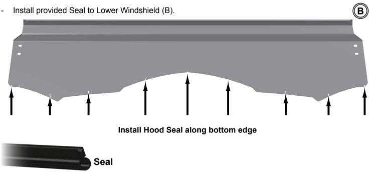
To ease installation, soak Seal in hot water before cutting or installing to increase flexibility.
