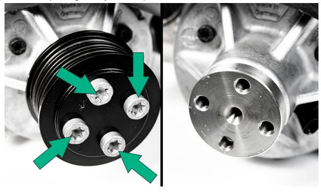
Install your new IE supercharger pulley and 4 included new bolts to the charger with a 6mm allen socket. Torque bolts to 23nm + one 90 degrees turn.
