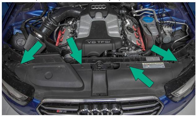
Remove the cowl carefully by pulling upwards.
