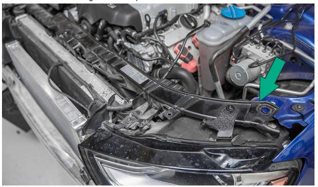
Pull to remove the engine cover plastic.
