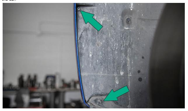
Pull the liner out of the way to gain access inside the fender. Remove the 10mm bolt directly behind the liner. Now loosen the two 10mm nuts under the bumper to fender bracket. You do not have to fully remove these nuts. *Repeat this step on both sides of the car.*
