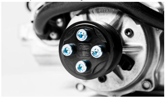
With the new pulley installed, reassemble the car by following the reverse of this procedure.
