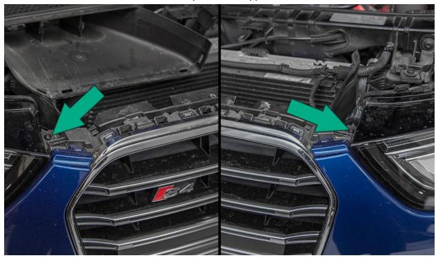
Release the bumper cover from the fender by pulling on the outer top edge. Repeat on both sides. *Note: Use caution during this step to not break the plastic clips that fasten the bumper.*
