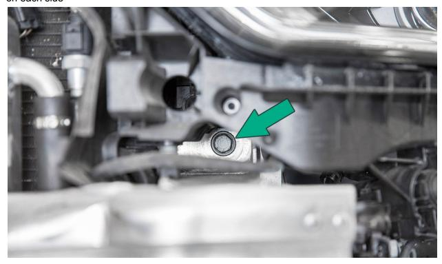
Remove the lower crash beam to radiator support bolts with a 16mm socket, two located on each side. *Note: We highly recommend installing a 10mmX1.5 threaded bolt at least 60mm in a lower hole on each side to support the weight.*
