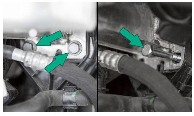
With the weight supported, carefully pull the front clip forward to access the pulley. Verify no lines or harnesses are being stretched or pulled.
