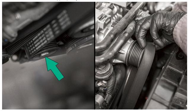
Using a T45 torx, remove the 4 supercharger pulley bolts and the factory supercharger pulley. (**Note:** Supercharger removed from the vehicle in photos to help with visuals only, do not remove the supercharger from your vehicle).
