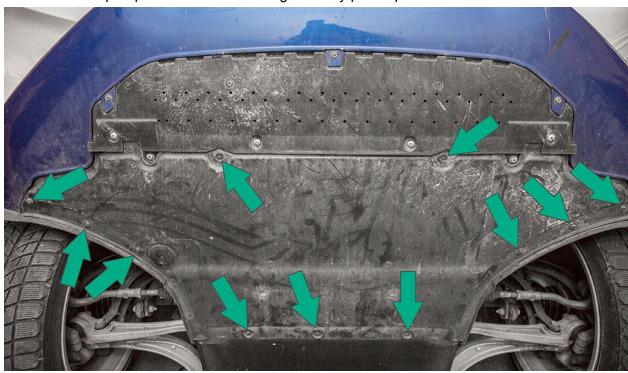
Remove belly pan from the vehicle by sliding backward.
