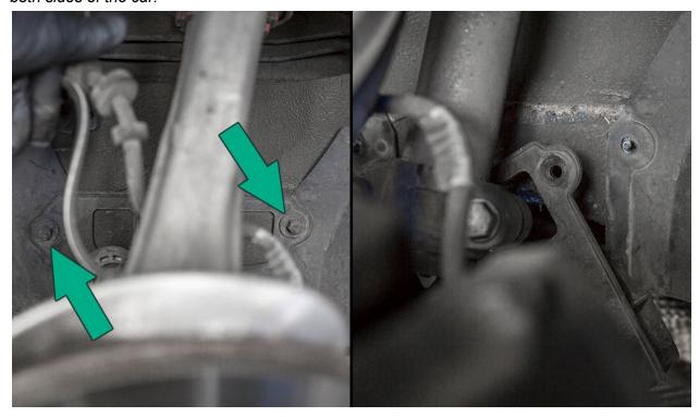
Using a small flathead, remove the two plastic retainers from the wheel well liner. Repeat this step on both sides of the car.
