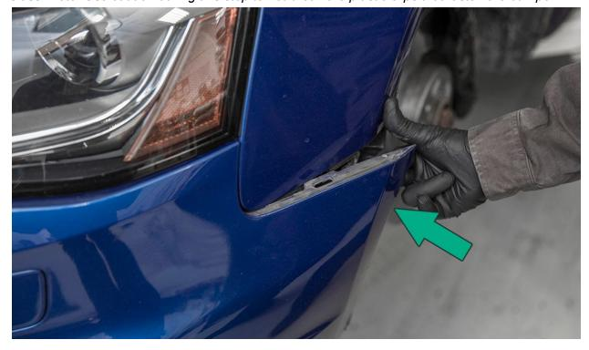
Pull the driver's side of the bumper cover forward and disconnect all electrical connectors located inside. *Note: Do not pull bumper too far forward in this step, it can damage the bumper harness.*
