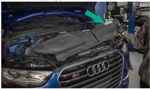
Remove the two T25 screws from the bumper to rad support, one on each side.
