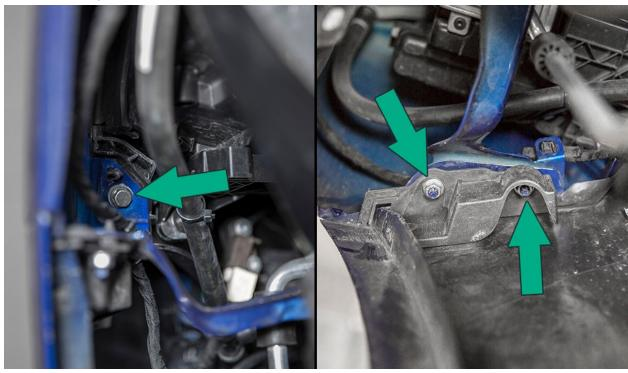
Remove the four push retainers or T30 bolts (varies by car) from the radiator cowl.
