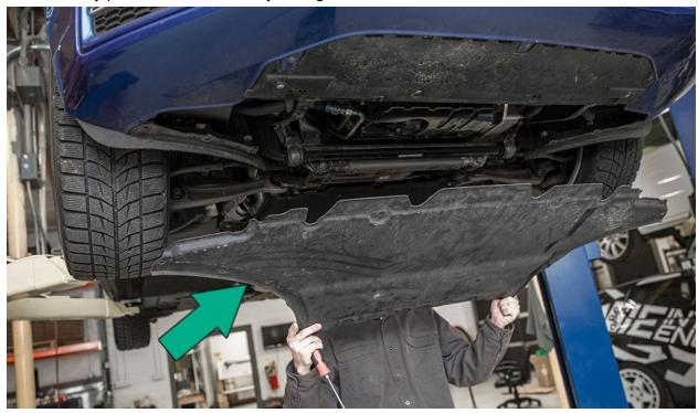
Remove the six T30 torx screws from the underside of the bumper that secures it to the radiator support.
