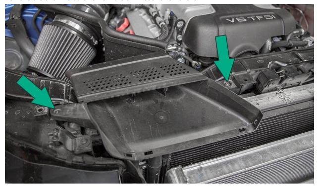
Remove the two T30 radiator support to fender bolts, one is located on each side above the headlights.
