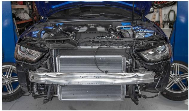
Remove the two T25 screws from the air inlet and remove it.
