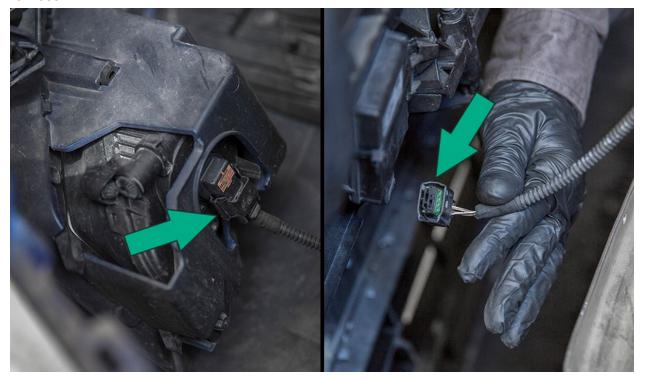
Verify all harness connectors are disconnected and free, then completely remove the front bumper.
