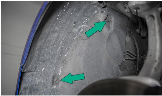
Remove the two outer T25 screws from the wheel well liner. Repeat this step on both sides of the car.
