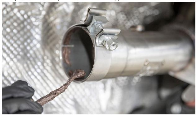
Slide the catalytic converter into the downpipe. Do not tighten exhaust clamp in this step.
