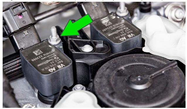
Using a T30 torx driver, remove the torx bolt from the PCV breather return hose.
