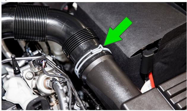
Using a T30 torx driver, remove the torx bolt from the rear of the turbo inlet pipe. Note: set this bolt aside, you will need to re-use it when installing your new IE intake.
