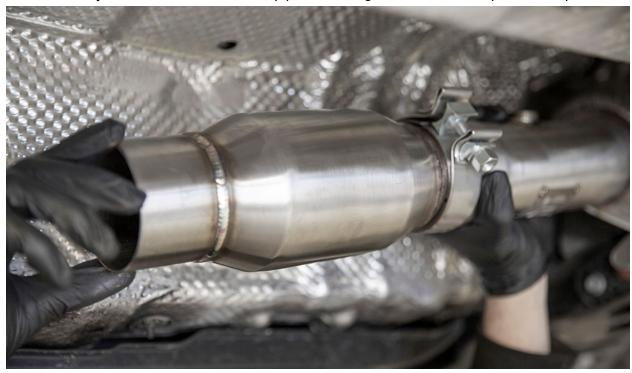
Loosely install the exhaust clamp and anti-seize onto the midpipe slip-fit end.
