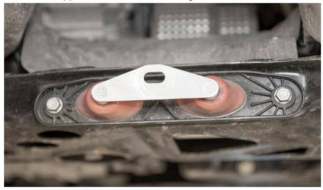
Carefully slide your new IE downpipe into place and install the included bolt, washers, and nut to the IE mount bracket finger tight. *Do not tighten the bolt in this step.*
