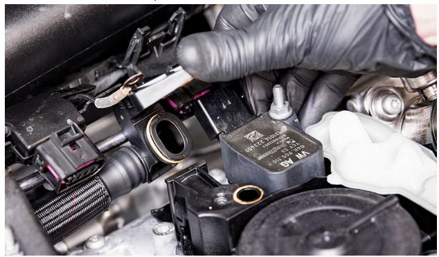
Using pliers or the factory hose clamp tool, release tension from the upper turbo inlet pipe coupler clamp and completely remove the turbo inlet pipe.
