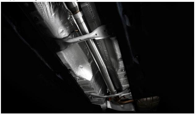
Verify all bolts and nuts are installed and tightened, all clamp connections are tight, make sure nothing is contacting the exhaust, and that your intake is fully installed. Start your car and inspect for any exhaust leaks. After driving the car for 1-2 days, verify all bolts, nuts, and clamps are tight, the exhaust is sitting straight, and there is no excessive pulling on any grommets. Enjoy the new sound and performance from your new IE performance downpipe!
