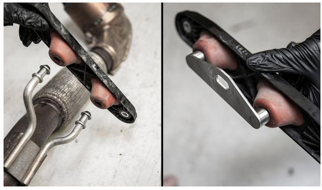
Reinstall the downpipe mount bracket to the vehicle using a 13mm socket.
