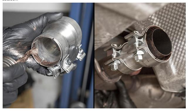
Loosely install exhaust clamp and anti-seize to the downpipe end.
