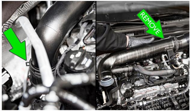
Loosen and remove the turbo v-band clamp bolt using a 6mm allen wrench and remove the v-band from the downpipe.
