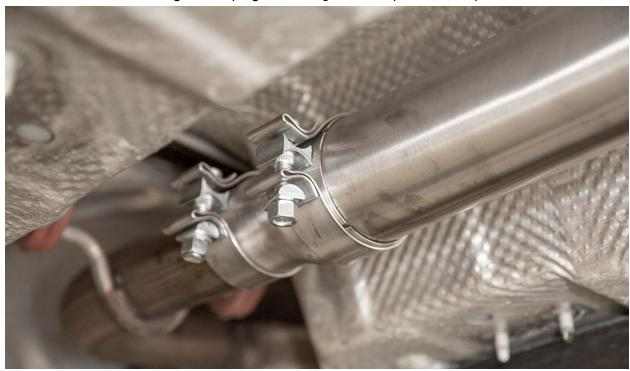
Align the downpipe with the turbo flange and reinstall v-band clamp then tighten bolt with 6mm allen.
