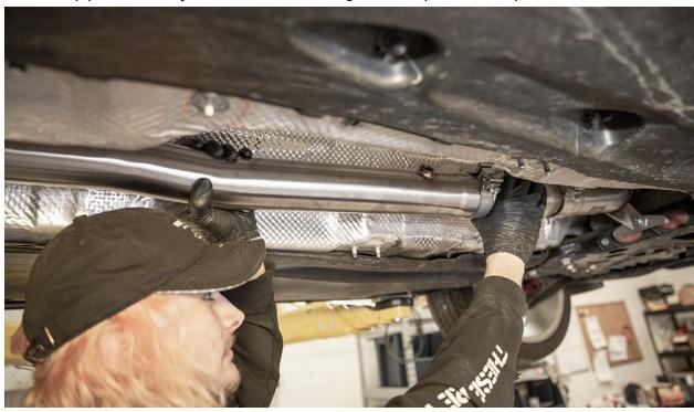
Slide slip-fit adapter onto the midpipe as far as possible. Adjust so that everything sits even, seated, and without binding or drooping. *Do not tighten clamps in this step.*
