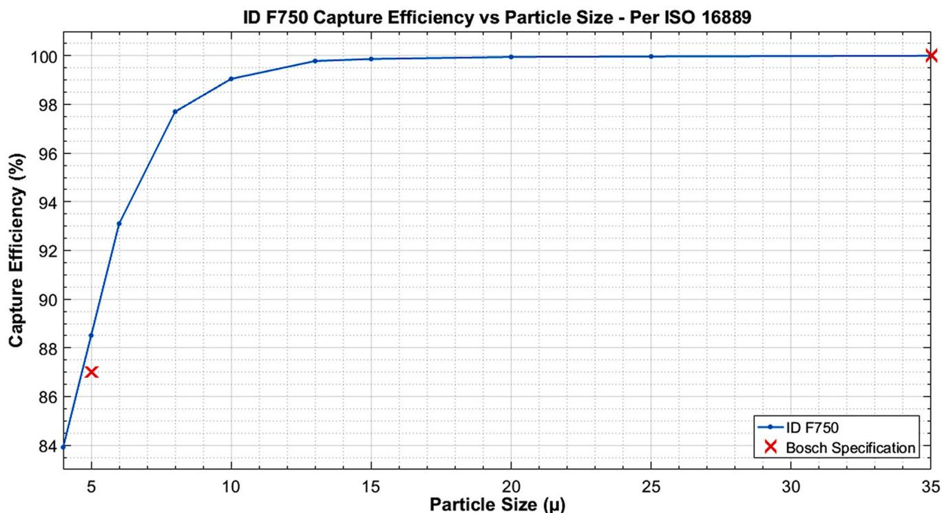
Note that for a filter specification to be meaningful, particle diameter and capture efficiency must both be stated. A nominal filter rating is useless, as it says nothing about the efficiency at the stated particle size.
