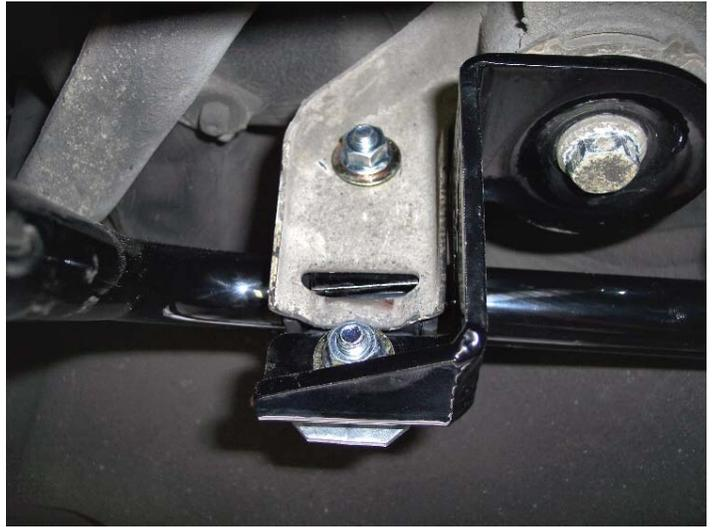
12R *Securing End Links to Sway Bar*
