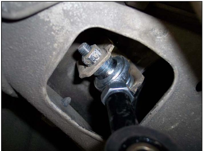
6R *Install the Bushing Mount Reinforcement Bracket*
