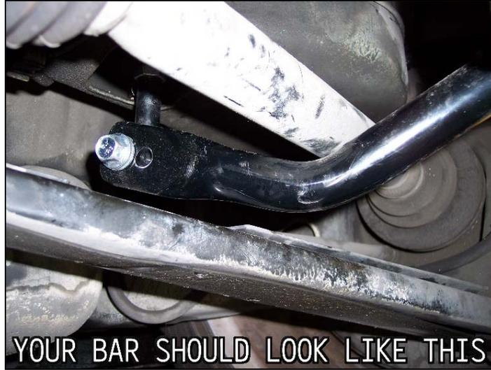
Once the gaps are equalized, grease the end link bushings and fully tighten the hardware including the jam nut that fastens the heim joint to the end link body.
