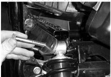
6) Once the bolt is through the bracket place two 10mm washers onto the bolt then insert the bolt into where the stock shock was located.
