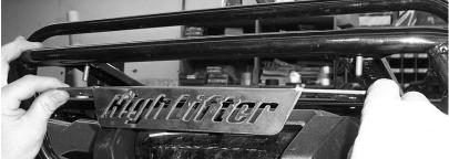
3. Secure the bracket using the  $\frac{1}{4}$  washer and  $\frac{1}{4}$  lock nut.
