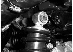
3) You need to take a look at the clamp that secures the exhaust to the ATV. You may need to rotate the clamp so that it does not come in contact with the top of the shock once the lift kit is installed. Loosen the clamp and rotate it down away from the shock. Once you have done this tighten the clamp.
