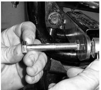
14) On either side of the shock eyelet you will need to place small spacers.
