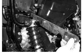
11) Loosely connect the bracket to the frame by placing it onto the bolts. Secure it with the 10mm lock nuts provided.
