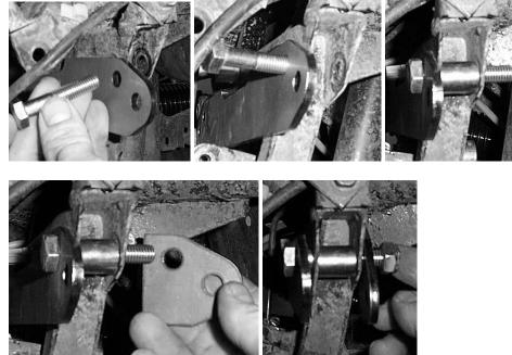
5) Next, connect the top of the shock to the lift bracket. Make sure to place a 10mm washer on either side of the shock eyelet. Secure it with a 10x50mm hex bolt and 10mm lock nut.
