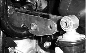
13) Insert a 10mm x 70mm bolt through the bracket.
