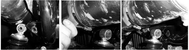
4) Insert a long rear lift bracket into the frame to the rear of the ATV. Make sure to insert with the cutout for the frame on the brackets are on the bottom.
