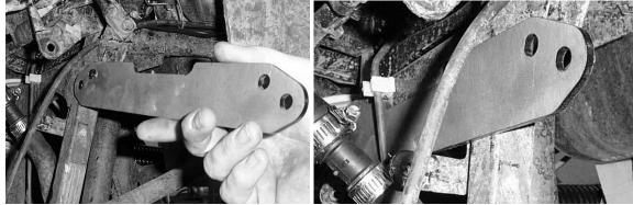
4) Place the Medium Spacer in the shock mount on the frame and connect the Small Front Lift bracket to the inside of the fame using a 10x50mm hex bolt and 10mm lock nut.
