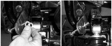
7) Insert a Large Rear Spacer into where the shock was located and push the bolt all the way through the spacer and out to the opposite side of the frame.
