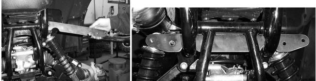
5) Insert into the bracket a 10mm x 70mm bolt.
