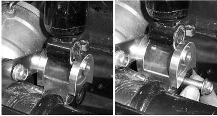
9) Connect the bottom of the shock to the lift block and logo bracket by using the 10x65mm bolt and 10mm lock nut provided.
