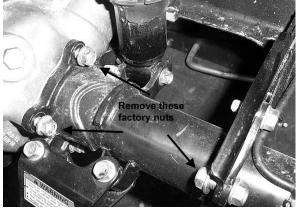
6) Place two 10mm washers on the bolts on the differential.
