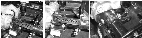
8) Next insert the rear lift block onto the shock mount. Make sure that the raised area on the outside of the lift block points away from the differential. Using the factory bolt and nut to connect the block to the shock mount.
