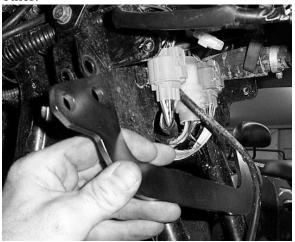
4) Place the Spacer in the shock mount on the frame and connect the Small Front Lift bracket to the inside of the fame using a 10x45 hex bolt and 10mm lock nut.
