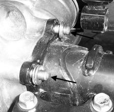
7) Now connect the rear logo bracket to the frame and differential. Secure it with the factory nuts that you removed earlier.
