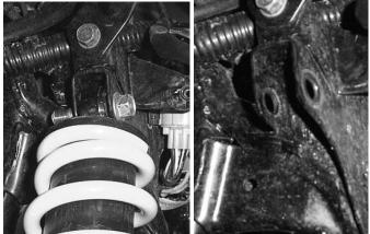
3) Insert the Long Front Lift bracket to the front of the ATV, running it from one shock mount to the other.
