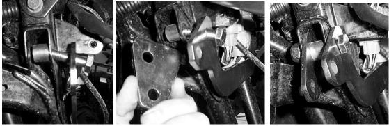
5) Next, connect the top of the shock to the lift bracket. Secure it with a 10x45mm hex bolt and 10mm lock nut.
