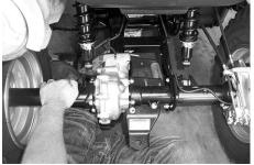
3) Remove two factory nuts from the rear. One from the left side of the differential and the other is to the right of the differential.
