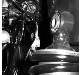
3) On the right side of the ATV, where the top of the shock connects to the frame there is a wire hook that holds a connecting clip. You will need to unhook the clip from the wire hook. With a pair of pliers, mash the clip flat.
