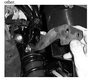
6) Place the Large Spacer in the shock mount on the frame and connect the Small Front Lift bracket to the fame using a 10x50 hex bolt and 10mm lock nut.
