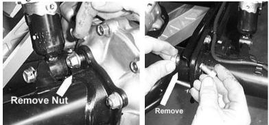
4) Next connect the Large Rear Lift Bracket and Small Rear Lift Bracket to the rear shock mounts. Using the stock bolt that connected the shock to the frame, connect the bracket to the frame. Place the Small Spacer between the shock mount tab and Large Lift Bracket. To the outside of the shock mount tab use the Small Rear Lift Bracket. **NOTE: The cut out on the small bracket clears the shock tab.**
