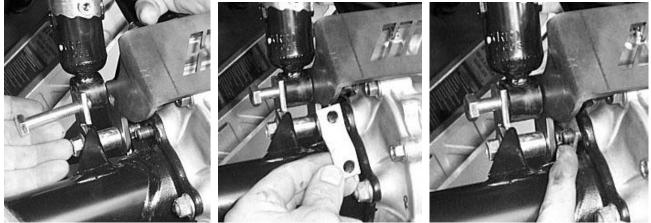
7) Right Side Installation: Using a 10x55mm hex bolt connect the shock to the bracket, placing the Right Rear lift bracket to the inside of the Large Lift Bracket. Secure it with a 10mm lock nut. Connect the Right Bracket to the bolt location where you had earlier removed the bolt and nut. Connect it with the factory bolt and nut.
