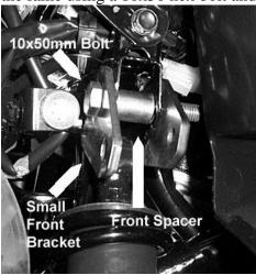
7) Next, connect the top of the shock to the lift bracket using 10mm flat washers on either side if the shock eye. Secure it with a 10x50mm hex bolt and 10mm lock nut.
