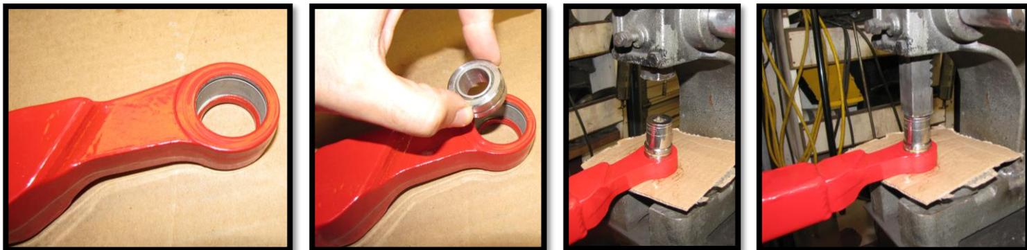
10. With the bearing seated all the way, you can now install the **100A** snap ring into the groove. If there's not enough room, you need to press the bearing in more.
