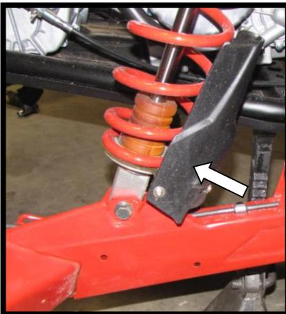
4. Disconnect the brake lines from the arms. You will need to drill out each rivet. Then retain your factory p-clips to reuse.
