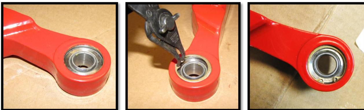
11. Insert a misalignment bushing **100F** into both sides of the bearing.
