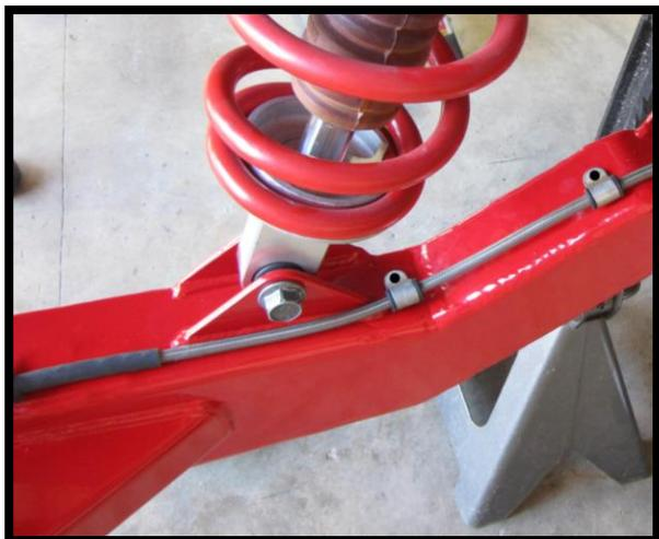
14. Connect the rear knuckle to the new trailing arm using the factory hardware.
