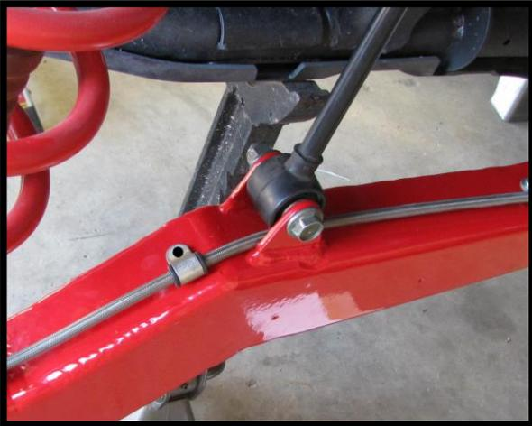
18. In the next steps you will attach the brake line by using the factory p-clamps, supplied p-clamps, and self-tapping screws into the holes already predrilled in the arms.
