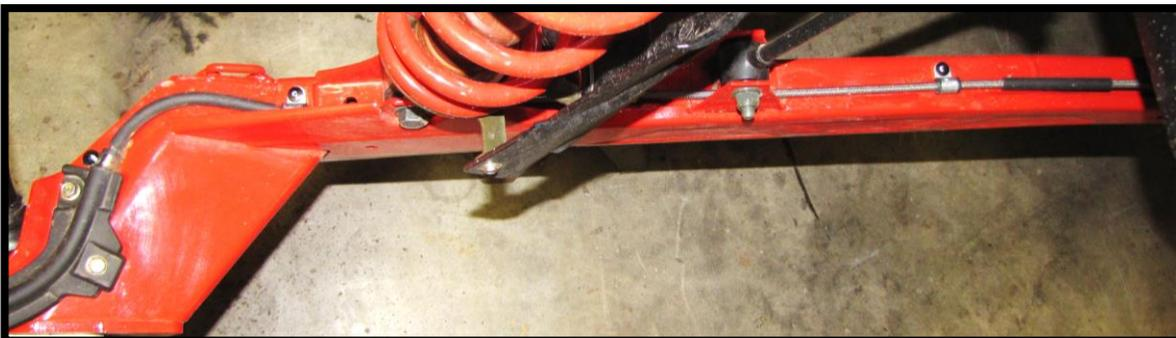
5. Disconnect the brake line guide/caliper/hub assembly/radius bars and knuckle from the factory trailing arms.
