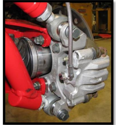
17. Attached the factory sway bar link to the new trailing arm using the factory hardware. Make sure the brake line runs under the sway bar link as shown below.
