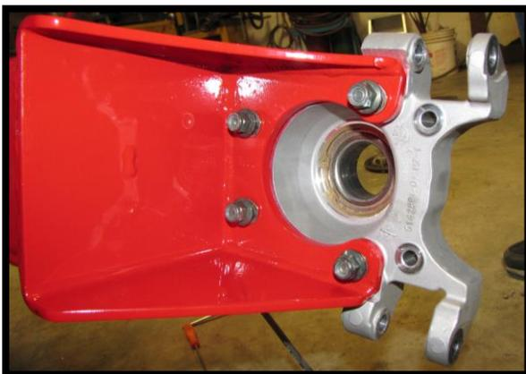
15. Insert the axle into the knuckle and install the radius bars using the factory hardware.
