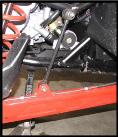
2. Next, jack up the rear of the UTV, securing it properly so that it does not fall, but it allows the arms to drop to full extension. Remove rear factory tires.
