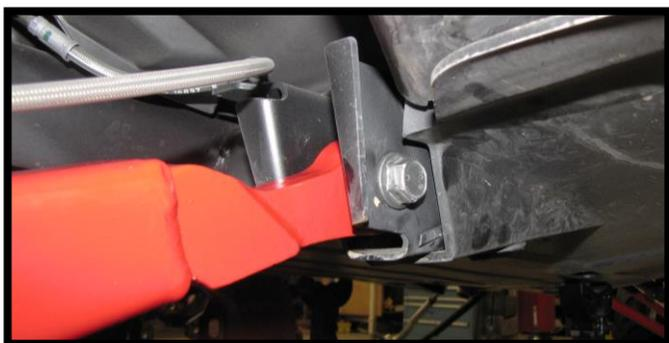
13. Connect the shock to the new trailing arm using the factory hardware. Make sure the brake line is to the outside of the shock tabs as shown below.
