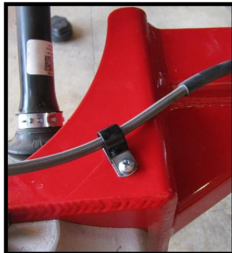
20. You will use your factory p-clamp next. The section of the brake line that has a strip of rubber surrounding it should line up with the next hole. If it does, you need to remove the piece of rubber that's inside your factory p-clamp and install the clip facing the correct direction as shown below. If it doesn't, then simply install it normally. Use a **#12-1" Tek self-tapping screw**. Do not over torque.
