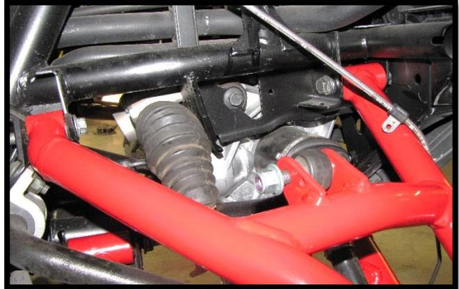
15. Reconnect the hub assembly, tie rod end, and sway bar link using factory hardware. Fasten to factory specifications.
