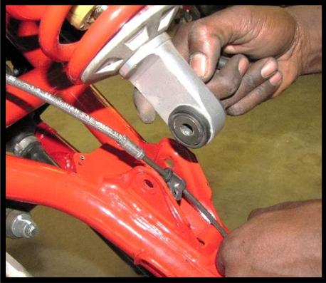
4. Disconnect the brake line from the upper control arm. You need to drill out each rivet until they break off.
