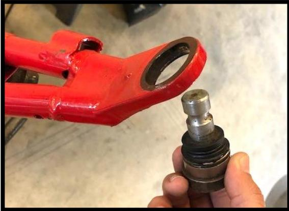
8. Before pressing the ball joints into the new High Lifter control arms, you may need to remove any built-up powder coating that could prevent the ball joint from seating all the way.
