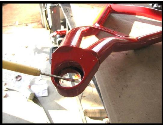
9. Install the ball joints into the new control arms.
