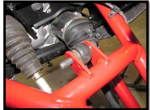
16. If you have not already done so, reconnect the bottom of the shock to the upper arm using the stock hardware. Fasten to factory specifications.
