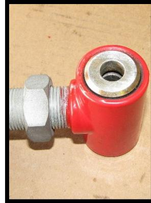
10. The new lower High Lifter control arms will already come adjusted to factory length. If you need to re-adjust the collars, place the arms on a flat surface. Measure from eyelet to ball joint on the factory arm, and then set adjust the new arm to those lengths.
