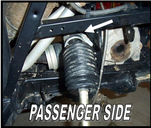
15. Next pull the boot back to expose the inner tie rod joint.
