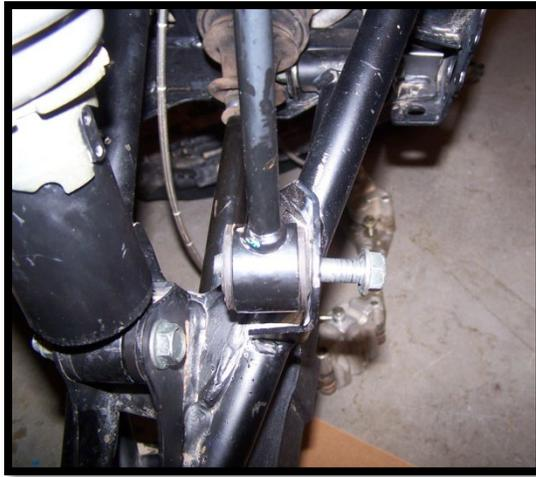
22. Reconnect the bottom of the shock to the upper arm using the stock hardware.
