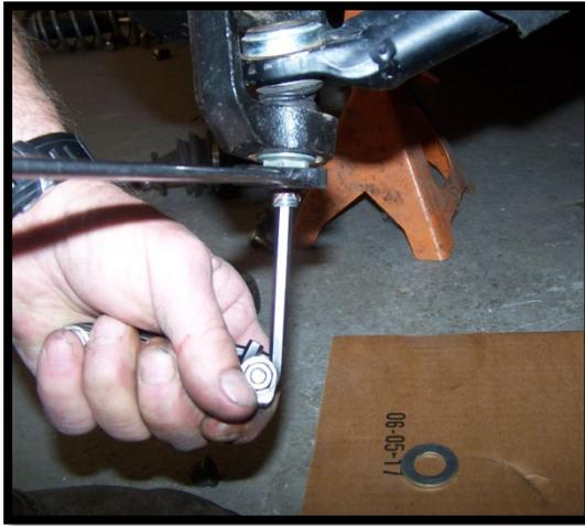
21. Reconnect the sway-bar to the upper control arm using the factory hardware.
