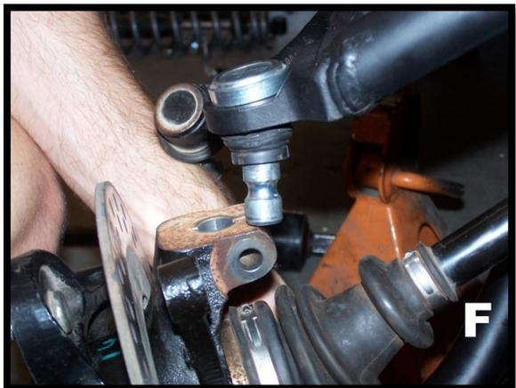
**NOTE: When disconnecting lower ball joint from the knuckle assembly. You will need a 6mm hex key to hold the stud in place while removing the nut.**
