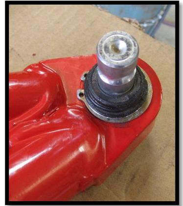
9. Now reinstall the bushings, sleeves, and pivot caps into the new arms. If you place some grease on them it makes the installation easier.
