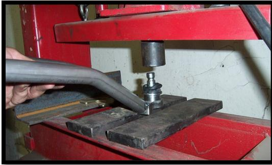
8. Reinstall ball joints into the NEW control arms.
