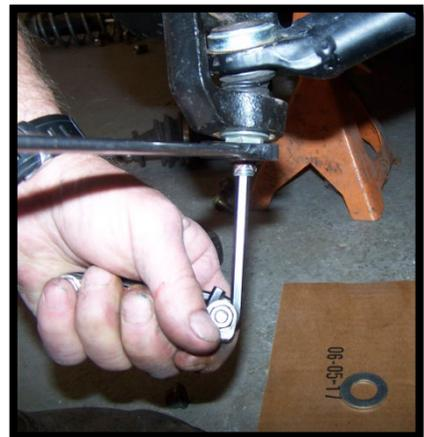
4. Now disconnect and remove the stock upper and lower control arms.(You will reuse the stock hardware)
