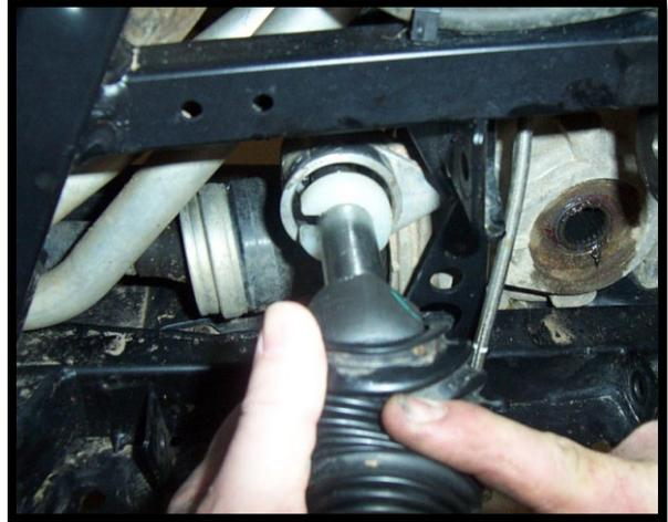
17. Pull boot back over the ball joint and steering stop and refasten with an (11" zip tie). Be sure to verify the zip tie is tight so prevent material from getting into the boot.
