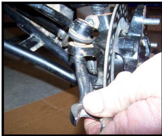
24. Reconnect the brake caliper and secure the brake line. Use the 8" zip ties provided to secure the brake line to the new upper control arm.
