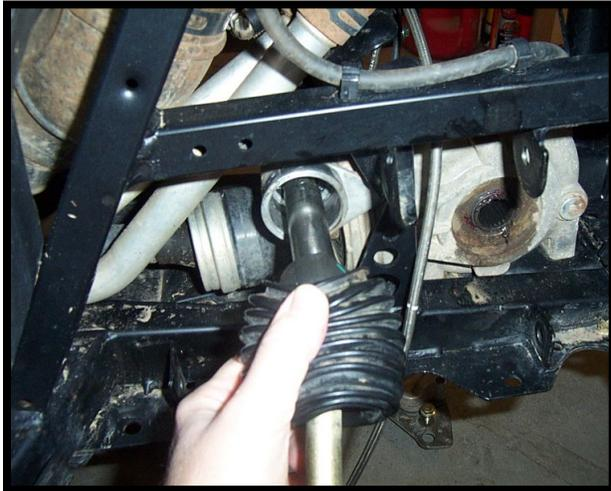
16. Place the steering stop (10U) clip between the inner tie rod joint and the rack and pinion. It is a tight fit, so you may have to force it on this is to ensure that the spacer stays in place.
