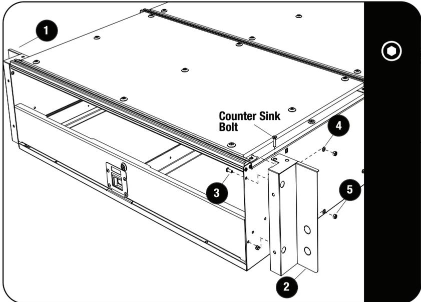
Loosen the counter sink bolt as shown. Secure the front faces (item 1 & 2) with item 3, 4 and 5. Refit the counter sink bolt.
