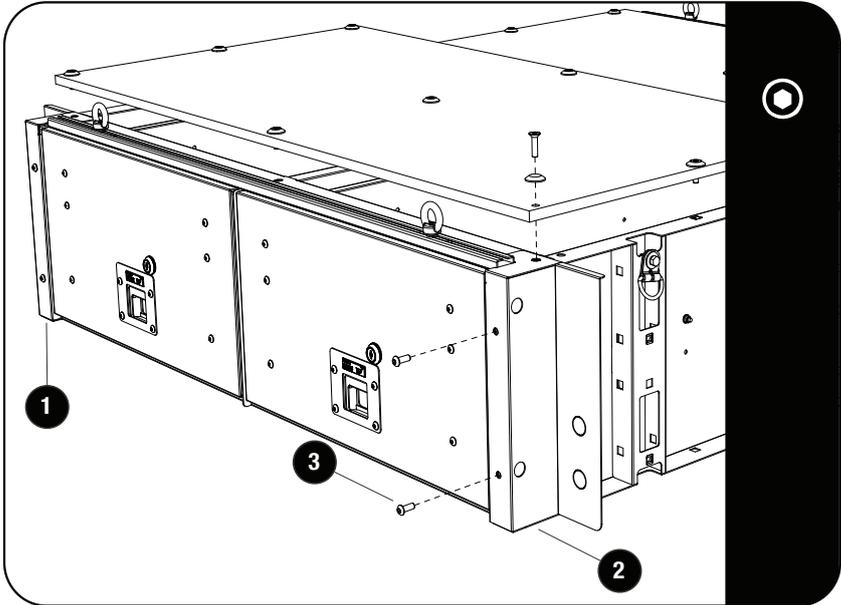
Loosen the drawer top as shown. Secure the front faces (item 1 & 2) with item 3. Refit the drawer top.
