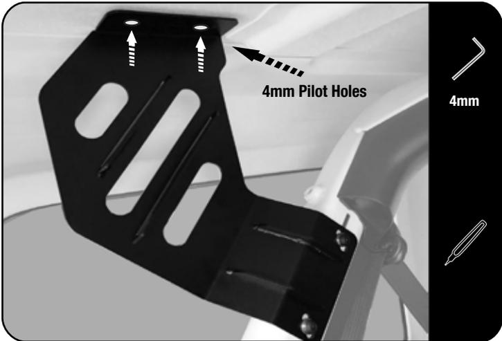
Fit the Inner Support Brackets (Items 6LH & 6RH) using the factory inserts in the roll bar, using M8 x 25 Button Head Bolts, M8 SS Spring Washer and M8 x 16 x 1.6SS Flat Washer (Items 16, 17 & 18). Refer to Figure 1.1 on page 3.
