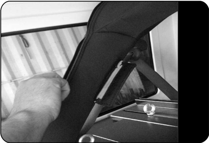
Loosen velcro, unzip and remove the padding covering the roll bars.
