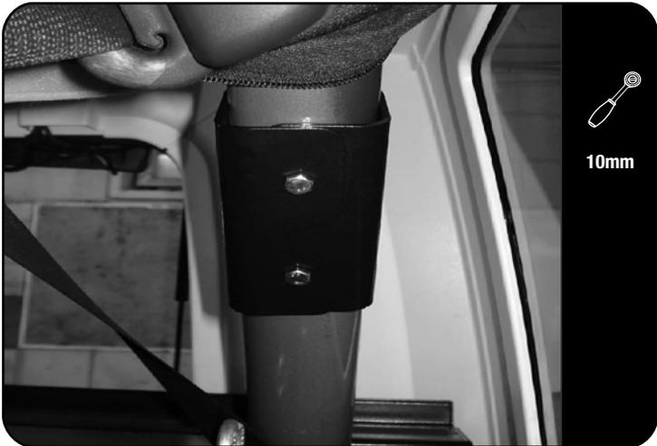
Locate the two threaded holes on the underside of the roll bar and fasten the two halves of the Roll Bar Clamps (Items 1 & 2) to the roll bar using M6 x 19 z 1SS Flat Washers and M6 x 20 Hex Bolts (Items 3 & 8). Place the Outer Roll Bar Clamp (Item 2) first followed by the Inner Roll Bar Clamp (Item 1).
