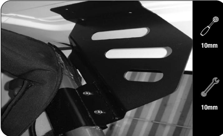
Recycling symbol: Refit and fasten the Rear Support Arms as in Step 2.3
