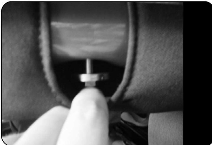
Pull back the padding around the roll bar above the rear seats and insert an M8 x 75 Hex Bolt and M8 Large Washer (Items 12 & 13 from FAJK002 box) through the hole as shown.
