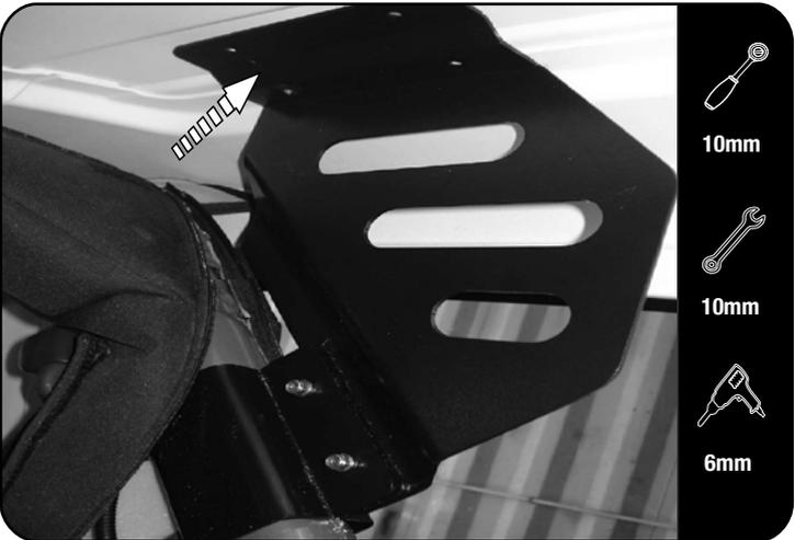
Loosely attach the Rear Support Arms (item 11) to the outside of the Roll Bar Clamps using items M6 x 20 Hex Bolts, M6 x 19 x 1SS Flat Washers and M6 Nyloc Nuts (Items 3, 7 & 8). Make sure the foot faces the inside of the vehicle and the contours of the foot match the contours of the roof as shown.
