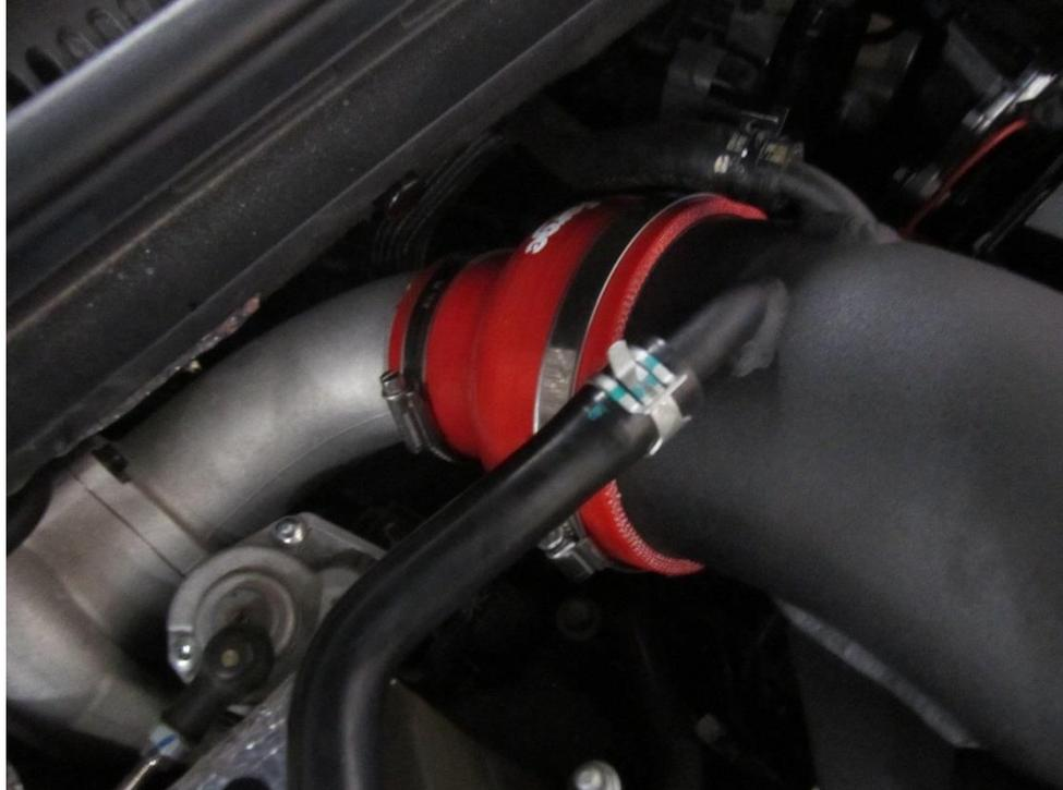
11. Re fit the engine cover locator through the intake pipe bracket. Now you can adjust the silicone hose and tighten it in position.
