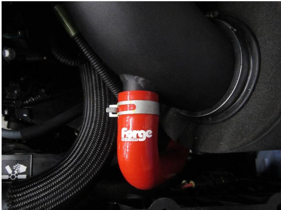
13. Finally, you may need to adjust the position of the air filter, just move into position so that it is not fouling or rubbing and then tighten the hose clamp. The installation of the Forge FMINDK28 is now complete, take your car for a test drive and enjoy.
