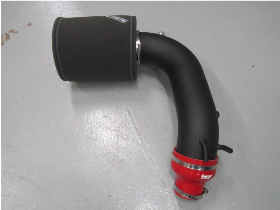
10. The intake can now be positioned in the engine bay, attach the silicone hose to the turbo elbow. Don't tighten the hose clamps at this point.
