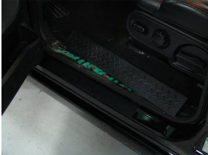
14. Loosen driver side A-pillar molding using your hands, and then remove the driver side lower kick panel.
