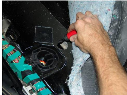
19. Recommended: Use a cotton swab or small brush to apply corrosion inhibitor to exposed edges.
