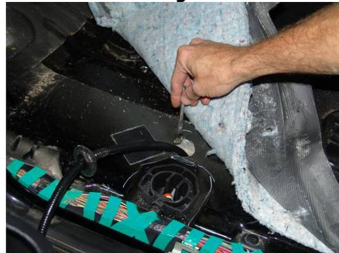
20. Route the supplied chassis harness through the drilled opening and seat the grommet from the inside of vehicle.
