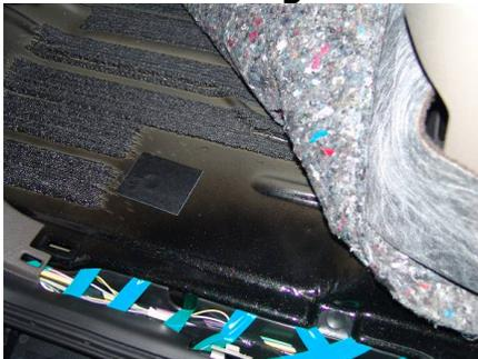
16. Secure F150 template over opening in front of driver's seat.
