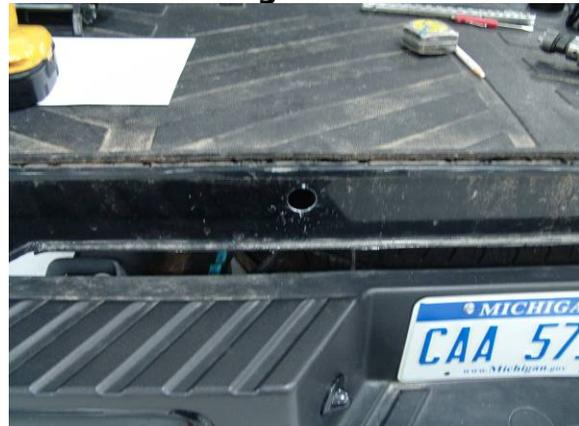
4. Clean the rough edges of the opening with a deburring tool. Recommended: Use a cotton swab or small brush to apply corrosion inhibitor to exposed edges (Figure 4). Reinstall tailgate.
