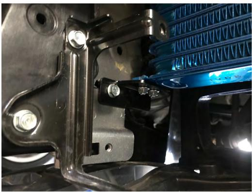
2.4 Connect the oil line between the sandwich adapter block fitting and the oil cooler. The 90deg fitting goes to the sandwich adapter block side and points down. The 180deg fitting goes to the passenger side (inner side) of the cooler and the 120deg fitting goes to the driver side (outer fitting) of the cooler. Route the line through the inner fender lining as shown in the picture.
