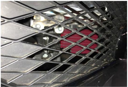
3.2 cut out the inner fender lining behind the oil cooler to get proper air flow behind the oil cooler. This can be done in various ways but if tracking the car, use wire mesh to protect the oil cooler core.
