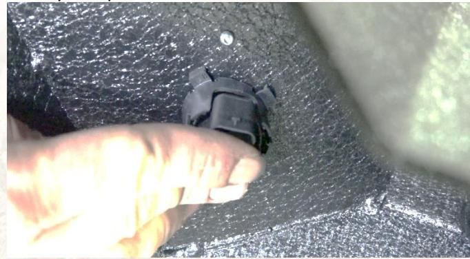
Remove the factory clip nuts from the JT's frame.
