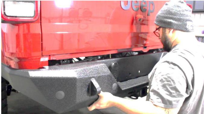
With the included flat washers, lock washers and hex nuts, secure the bumper to the left and right frame mounts with an 18mm Socket.
