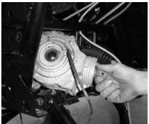
14) See the illustrated area in the photo below that need to be trimmed to allow access and fit of the differential and differential plate. The view is looking up from under the Ranger.
