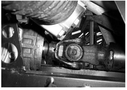
25) Connect the differential to the mounts on the plate. You will use two 10mm x 40mm bolts on the short mount and 10mm x 50mm bolt on the taller mount. **Make sure to use the Red thread locker provided on these bolts.**
