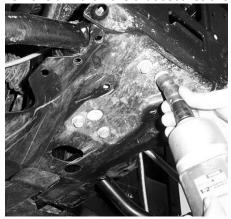
13) Remove the differential from the frame.
