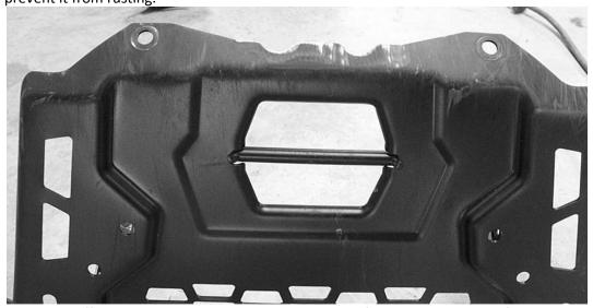
20) Insert the differential mounting plate into place on the frame by sliding it up from underneath. The taller differential mount goes towards the front.
