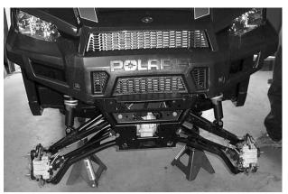
3) Disconnect the bottom of the front shock from the control arm.
