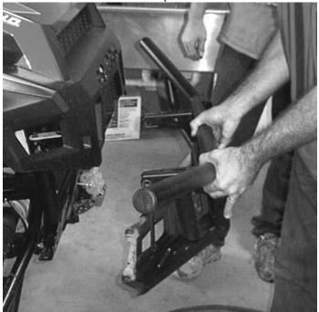
34) Where the bumper connects to differential plate, use the 10mm x 35mm bolts, 10mm flat washers and 10mm lock nuts.
