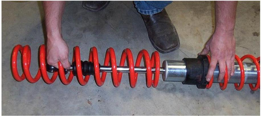
7) Now place the rear spring spacer on the shock.
