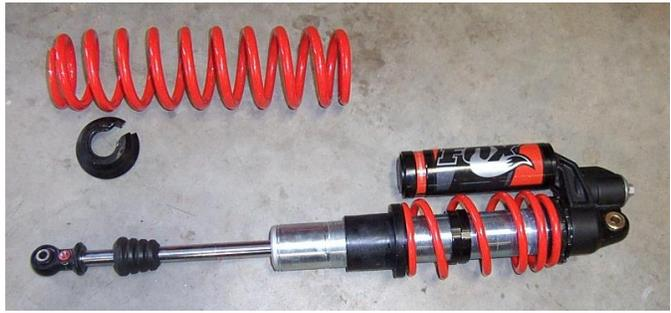
6) Place the front spring spacer to the shock.
