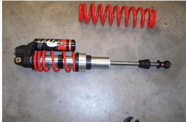
7) Reassemble the shock by placing the factory spring and retaining clip back onto the shock. You will need to compress the factory spring to reassemble. With the added height of the spring spacers, it requires compressing the springs to reassemble the shock.
