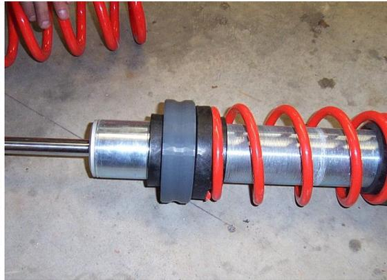
8) Reassemble the shock by placing the factory spring and retaining clip back onto the shock. With the added height of the spring spacer, it requires compressing the spring to reassemble the shock.
