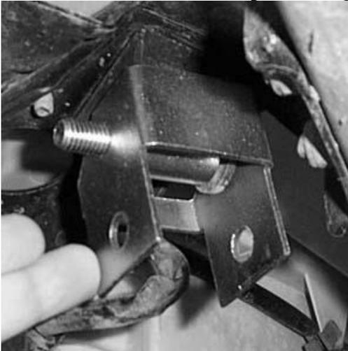
5. Insert the small spacer and top of the shock in the bottom of the lift racket.
