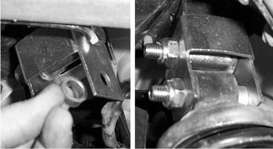
6. Secure the shock, bracket, and small spacer using the 10x60 hex bolt and 10mm lock nut.
