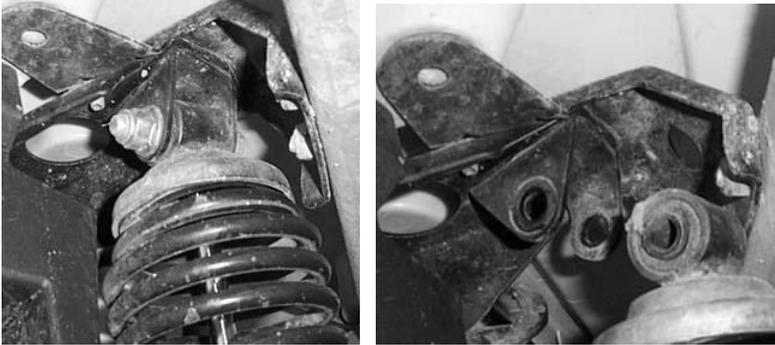
3. Install large spacer and front lift bracket into the upper stock shock mount location.
