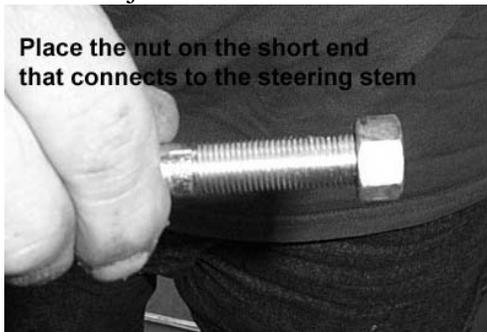
22) Now connect the joint and jam nut that was connect to the knuckle assembly to the longest end of the new tie rod.
