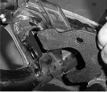
12) Insert the rear spacer into the shock mount tab next to the bracket, and then insert the 10x55.
