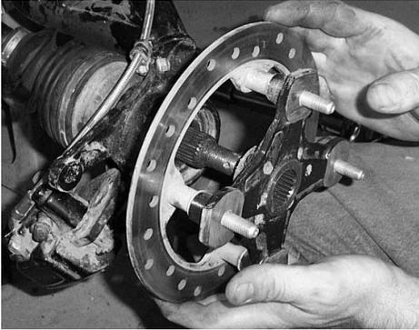
6) Disconnect the pivot rod. You only need to remove the nut from one side on the pivot rod. You can pull it out from the opposite side that has the nut still attached.
