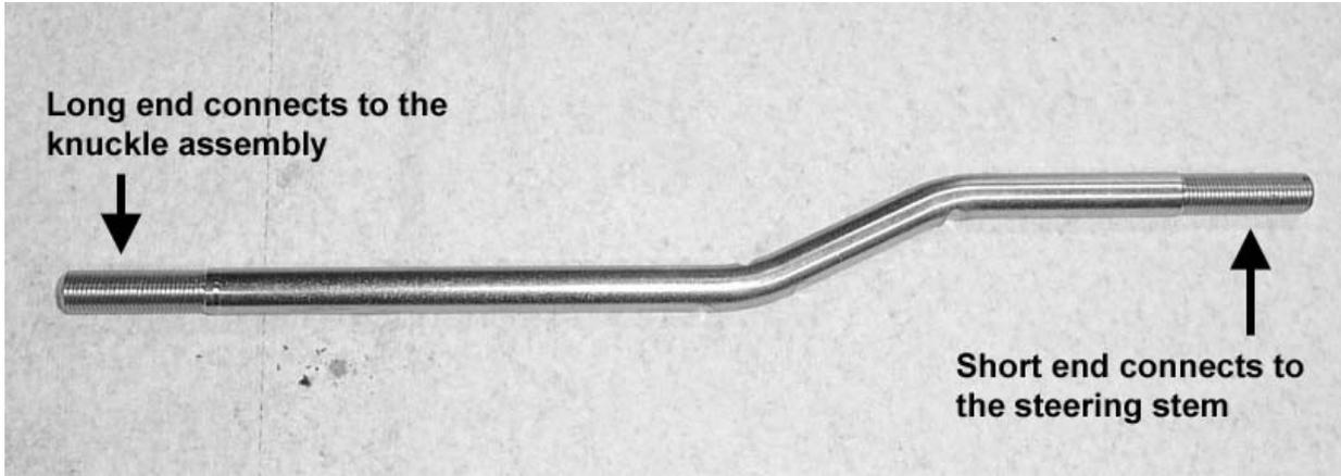
21) Place the jam nut that was connected to the steering stem to the short end of the new tie rod.
