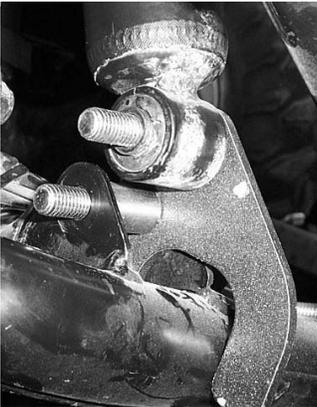
14) Place the other rear lift bracket to the outside of the shock tab and secure it with two 10mm lock nuts.
