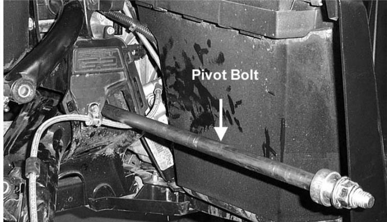
7) Once you remove the pivot rod the rear arms will be free from the ATV. Remove them then trim the marked area on the plate.
