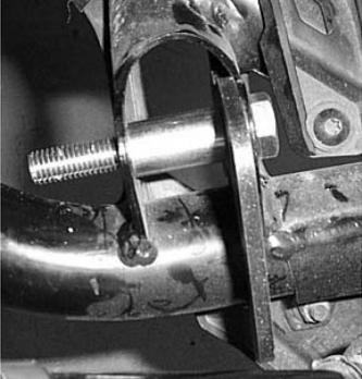
13) Connect the bottom of the shock to the lift bracket using a 10x55 hex bolt and 10mm lock nut.
