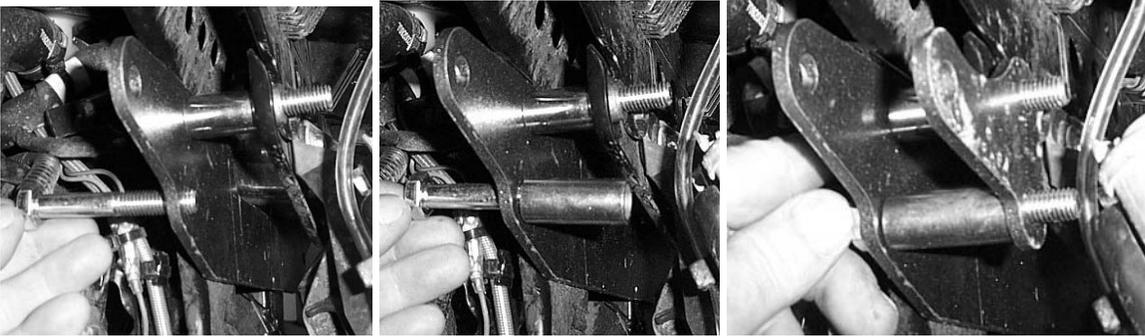
13) Loosely connect the brackets with the 10mm lock nut.
