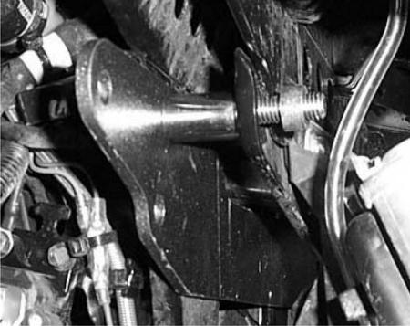
12) Insert a 10x65mm hex bolt into the lift bracket, then place the front large spacer on the bolt then place the small front lift bracket on both bolts to the outside of the shock mount tabs.
