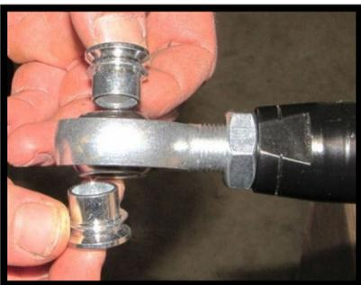
18. Slide a **12mm flat washer** onto a **1/2" x 2-3/4" bolt**. Insert it through the tabs and heim. Secure it with a **12mm flat washer** and **1/2" lock nut**. Torque the nut to 110lb-ft. Repeat to other side.
