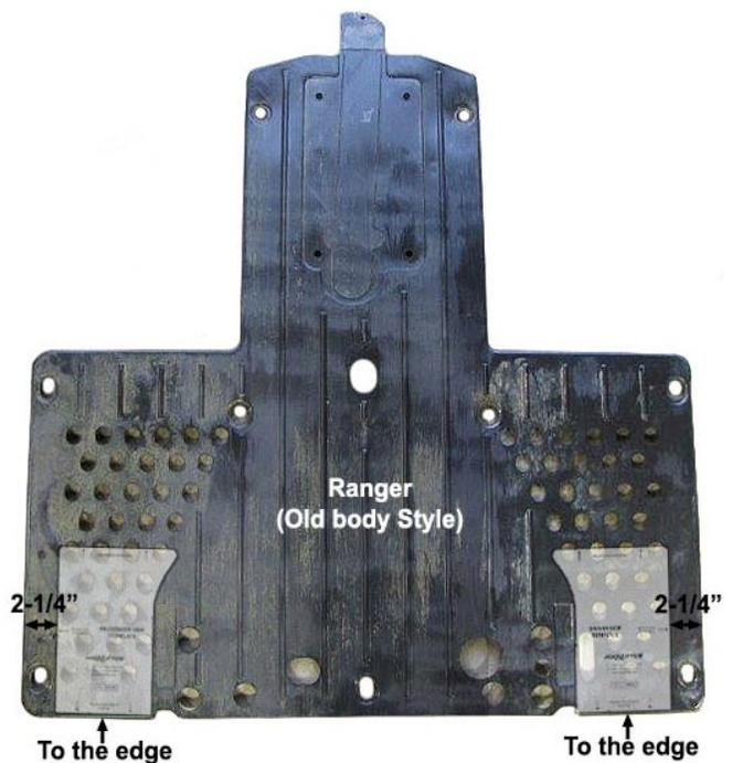
12. Cut the marked sections in the skid plate using an oscillating/cutting tool.
