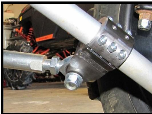
26. Next, you must complete a **CLEARANCE CHECK**. Follow the steps and check for clearance before riding. If you check before riding you can adjust before you damage the bars, clamps, or other parts.
