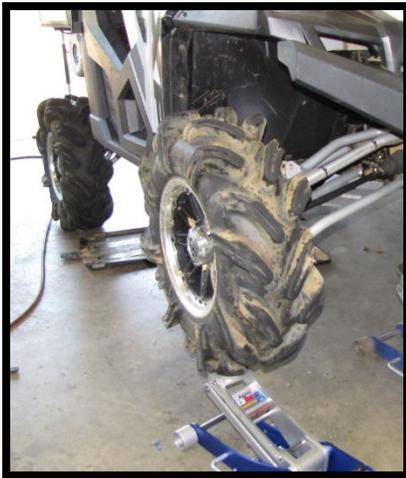
35. When the control arms are set to the fully compressed length, check to make sure that the adjustable link bar clears the frame.
