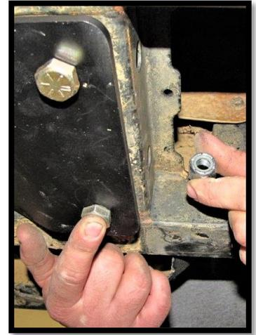
6. Using the three holes at the other side of the plate as a guide. Drill through them into the frame with a **5/16 drill bit**.
