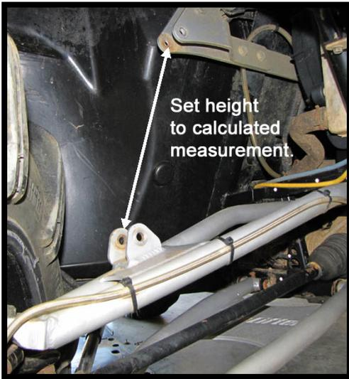
34. Use a jack stand or a friend to hold it in place while you situate the link bar to be close but not touching the frame. You can adjust the bars, slide the clamp up and down on the control arms, and rotate the collar to achieve proper clearance.
