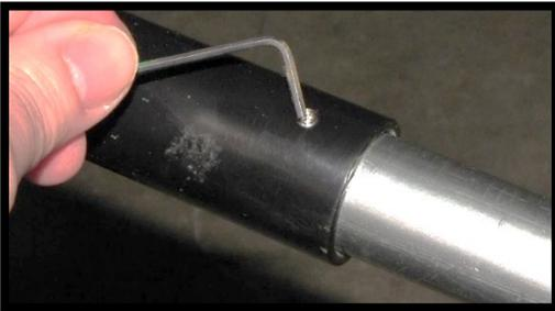
41. Located on each clamp collar are two ¼-20 x 3/8” set screws. Make sure that the set screws are tightened so that the collars cannot move during use.
