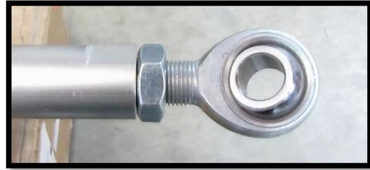
24. Adjust the inner bar so that the heim will reach the clamp collar tabs. Then insert (2) alignment cones 96Q into to the eyelet of the heim joint.
