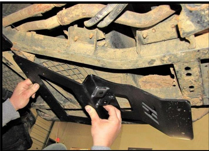
5. Slide a **1/2" flat washer** onto (2) **1/2" x 1" bolts** to connect the plate to the frame. Loosely secure them with **7/16" flat washers** and **1/2" lock nuts**.
