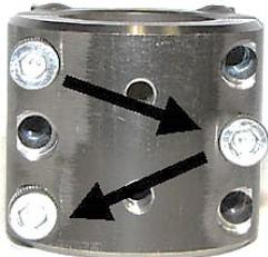
21. Loosely connect the **clamp collars 96R & 96T** onto the lower control arm. Connect it at the lowest point possible on the arm using the **1/4-20 x 3/4" socket head bolts**. **Keep in mind you will need to adjust it later, so fasten snug, not all the way tight.**
