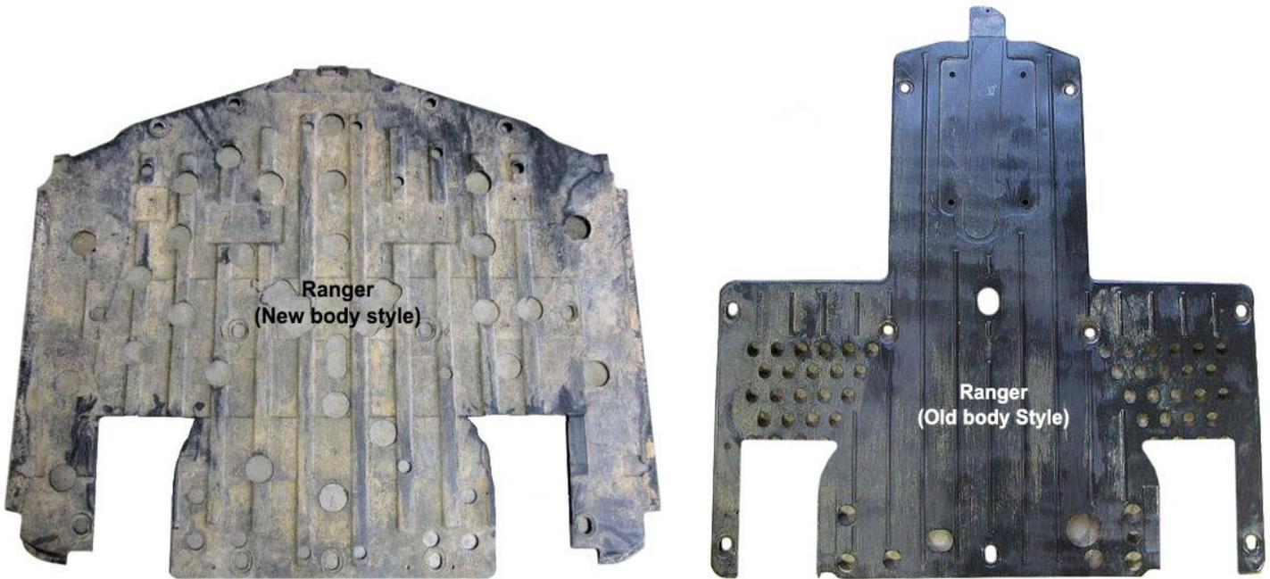
13. Reattach the skid plate over the control arm link plates. Re-secure the skid plate using the factory hardware.
