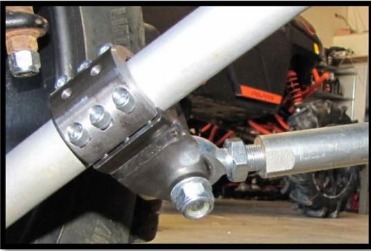
40. Located on each (hollow) bar is a single ¼-28 x 3/16” set screw. Make sure that the set screw is tight so that the bars will not rotate during use. Do not over torque.
