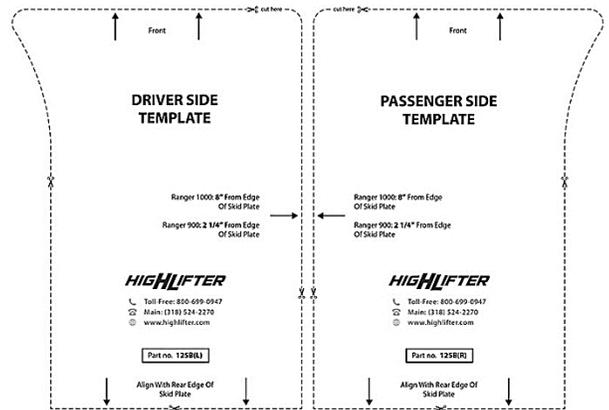
11. With the skid plate lying flat with the frame side down, place the templates down and follow the directions.
