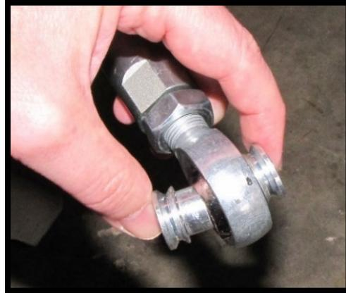
25. Connect the heim joint to the collar on the control arm. Slide a 12mm flat washer onto a ½" x 2-3/4" bolt. Insert it through the clamp collar and heim. Secure it with a 12mm flat washer and 1/2" lock nut. Torque the nut to 110lb-ft. Repeat to other side.
