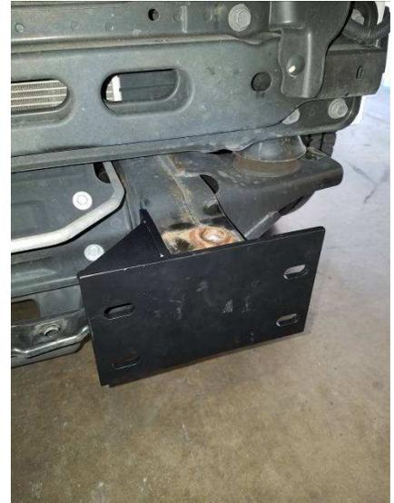
**Figure 9b.** Driver side steel mounting bracket.
