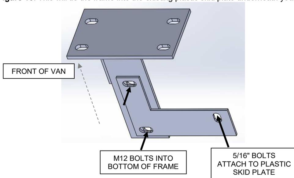
13. Use the factory tow-hook bolts OR the provided M12-1.25 bolts and 1/2" washers to thread through the bottom of the brackets and into the vehicle frame.
