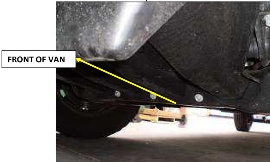
**Figure 3.** 6 bolts attaching the skid plate.
