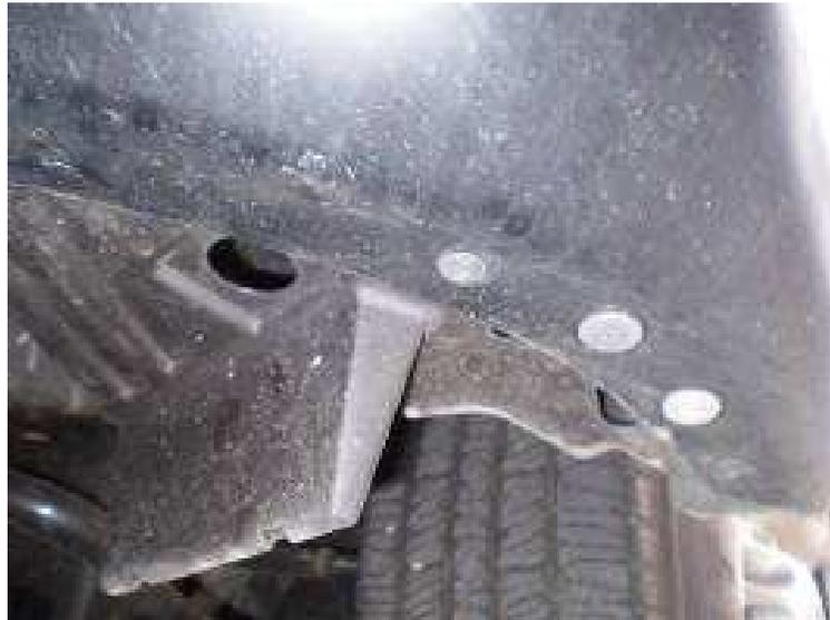
**Figure 1.** Remove 7 screws attaching the inner plastic fender.
