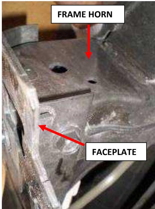
**Figure 7.** Remove faceplate before cutting welds on crossmember.
