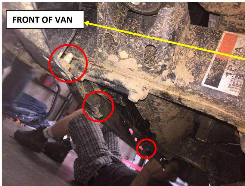
**Figure 4.** Bolts fastening the bumper to another support piece (4<sup>th</sup> bolt not pictured, out of frame to the left of the image)
