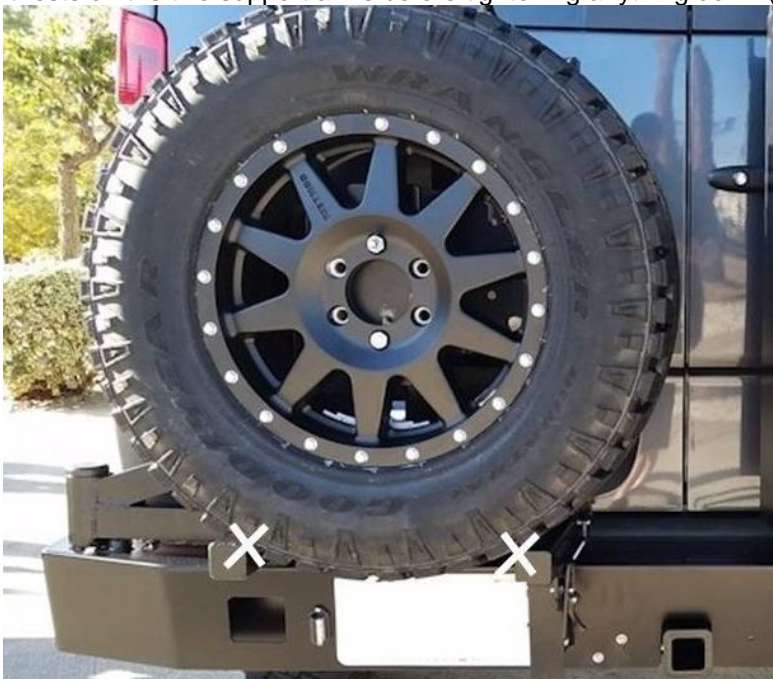
Figure 1. Rest tire on both support arms (before tightening the lugs or ubolts down). *NOTE* Your bumper may look different than the one seen in the above picture.
