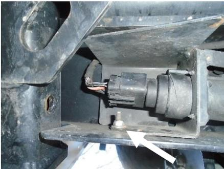
**Figure 5. Tow Plug with 1/4" button head screw.**
