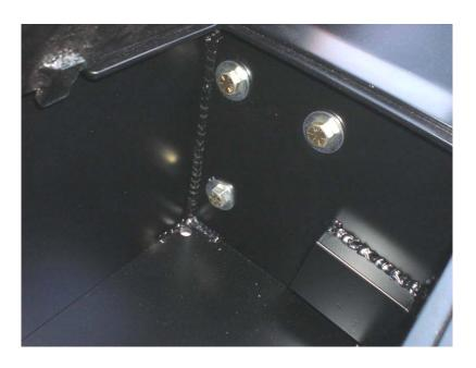
Figure 6: View of toolbox inside, showing correct orientation of mounting hardware
