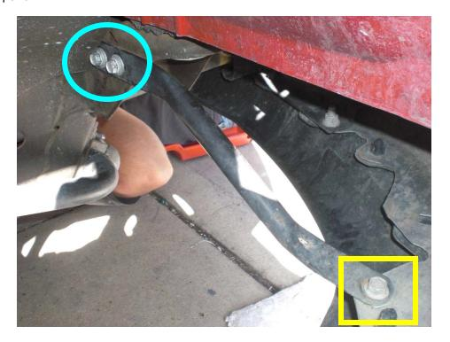
Figure 1: Stock bumper tension rod
