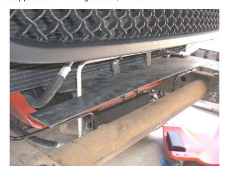
Figure 3: Trimmed plastic shield
