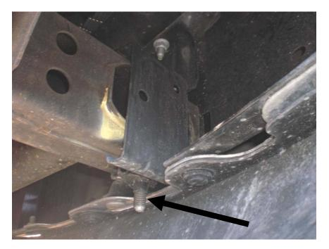
Figure 2: Stock bumper vertical retaining bolt
