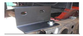
Figure 4: Installed bumper bracket
