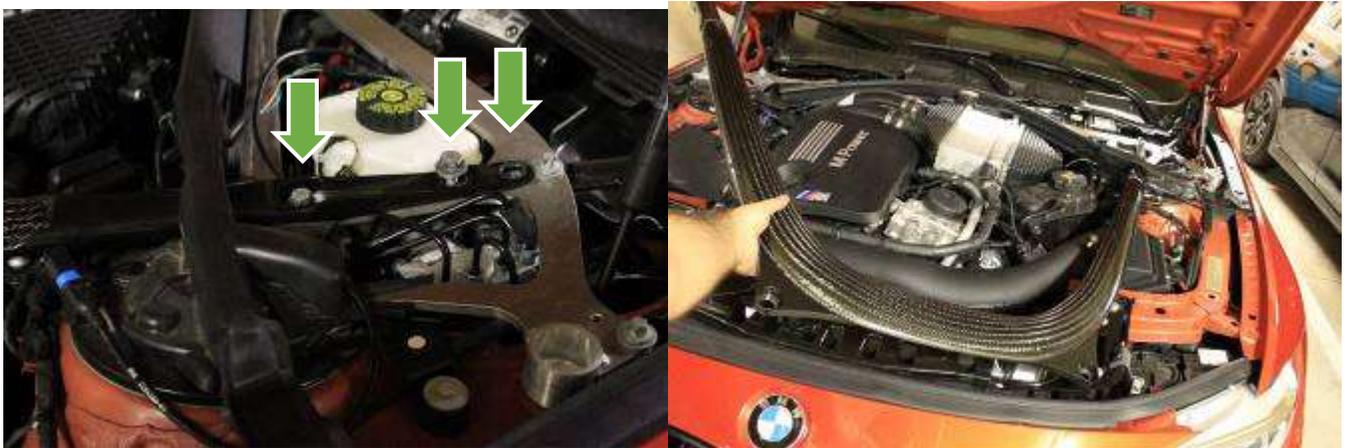
Remove passenger side airbox top and bottom.
