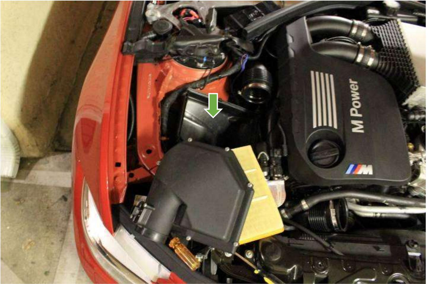
Remove the turbo inlet coupler
