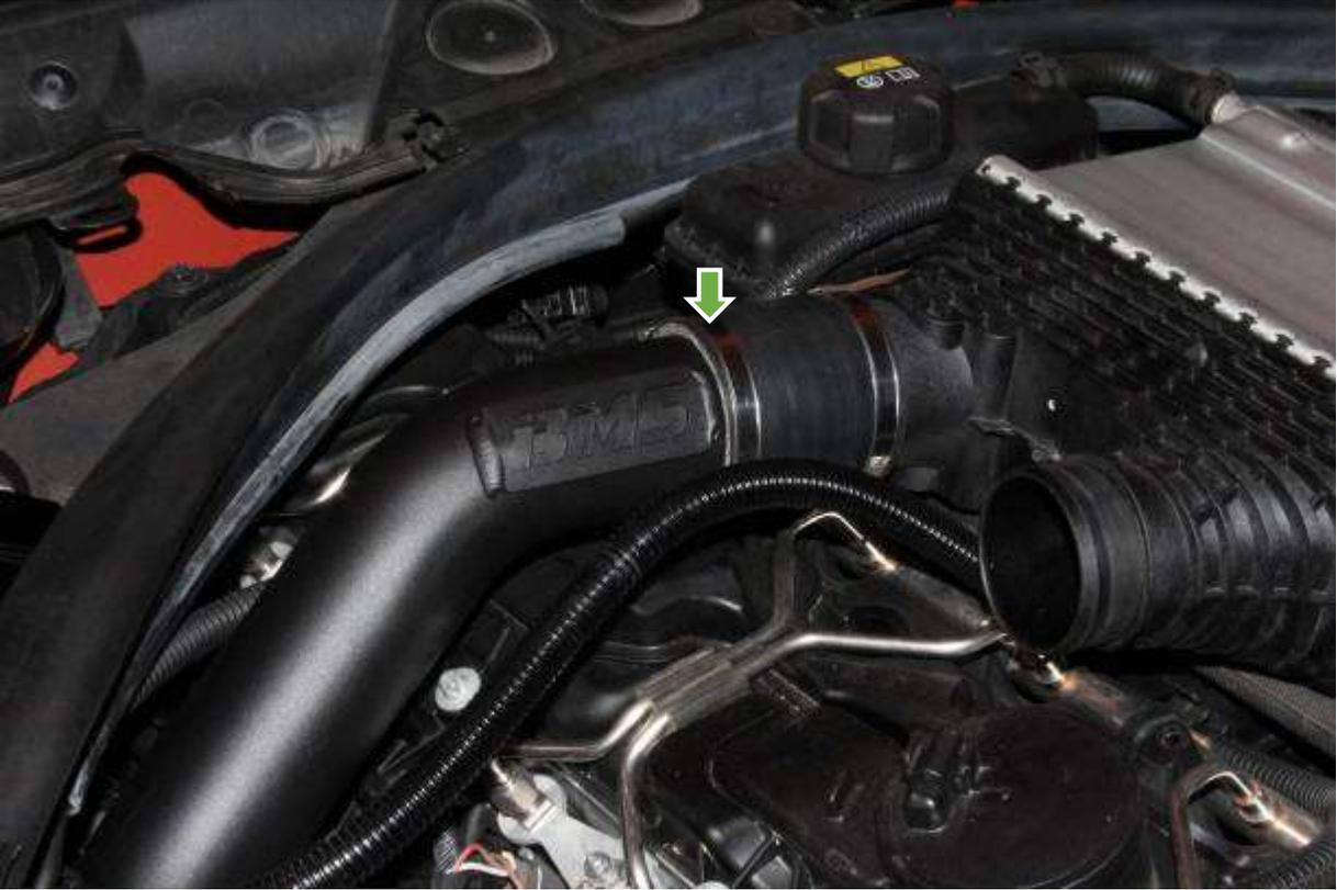
Now install back intake tube on the turbo.
