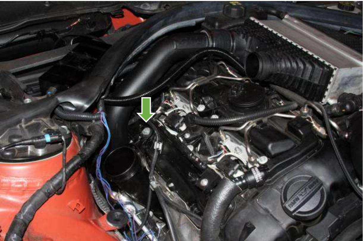
Install front chargepipe following the same steps as the rear pipe.
