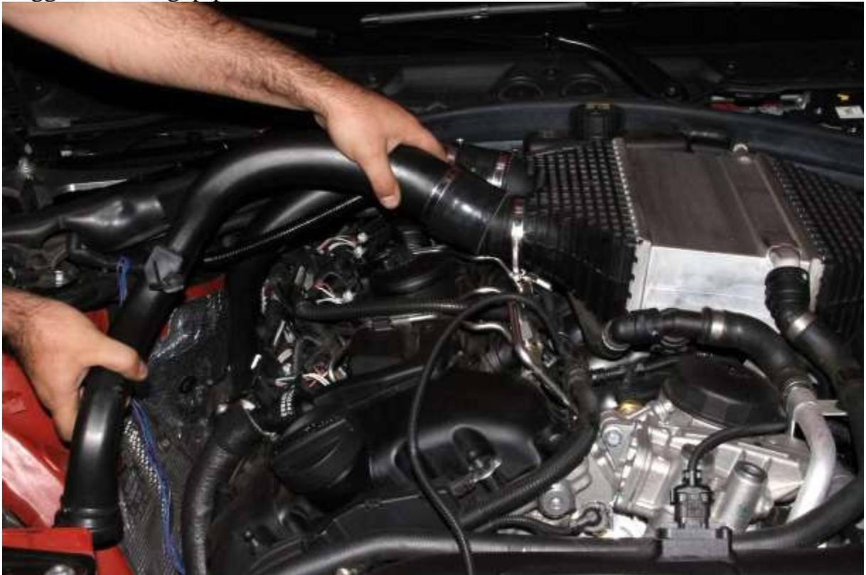
Remove O-ring from OEM chargepipes and transfer to BMS chargepipes.
