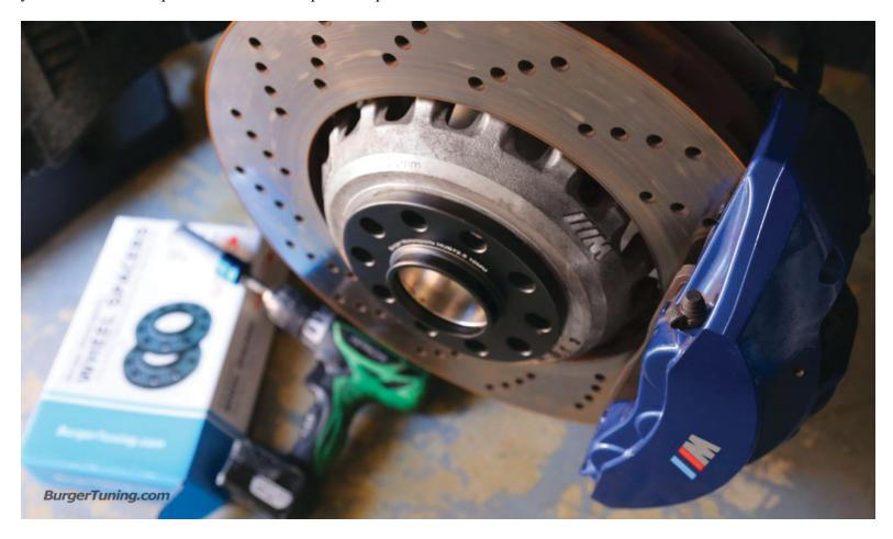
7. Use the correct length extended bolts that came with the spacers. Each spacer width has specific length bolts. Be sure not to mix them up if you have multiple spacer kits.
