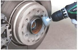
4. Don't coat the bolts or back of the spacer with anything (grease, anti-seise, etc) We supply a small packet of anti-seize for the top and sides of the factory hub and the spacer hub. This will aid in removal of the spacer. There are also pry tabs on the back of our spacers for easy removal.
